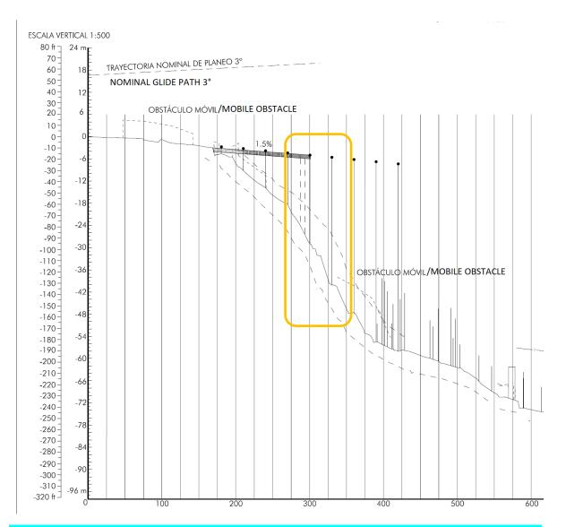
Figure 1: Typical example of 'very complex' with greater than 6 m 'sea wall' at 300 m (Asturias, LEAS 29 dated 2007) that after suitability assessment and due to the present of ARAS it may be changed to **'moderate'**.
