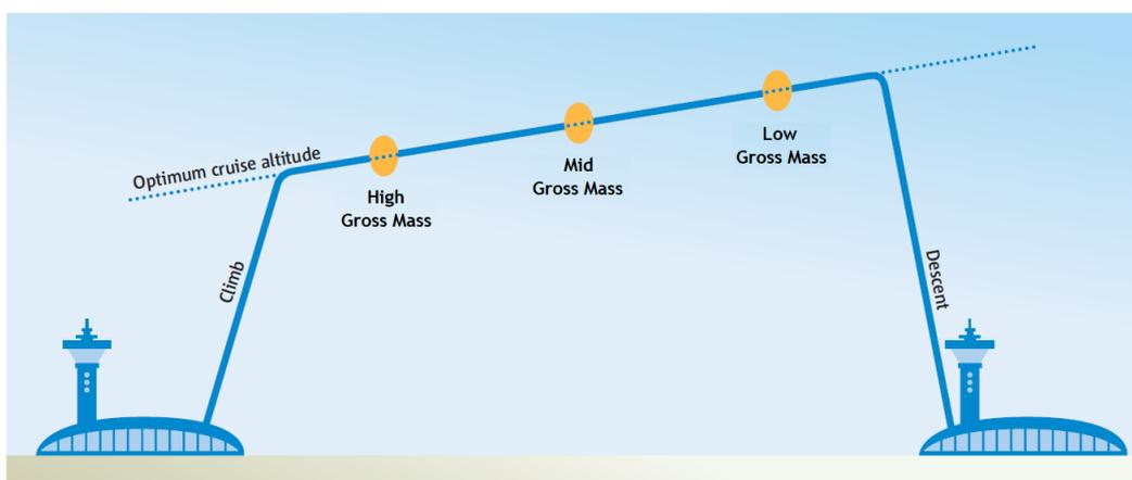
Figure 2 — Illustrative example of the three SAR measurement points for CO<sub>2</sub> emission evaluation
