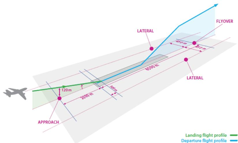
Figure 1 — Schematic of LTO noise certification measurement points
