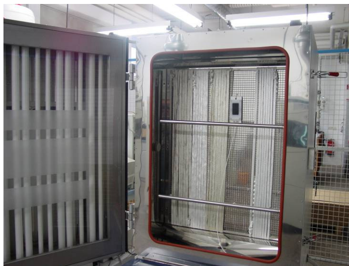
Figure 2: UV-Chamber at STFI – simulation of climate
