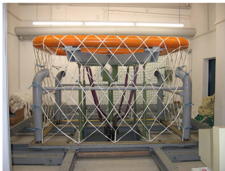
Figure 12: Test set-up for air cargo nets (size 96"x125"x118") at STFI e.V., (full scale test)
