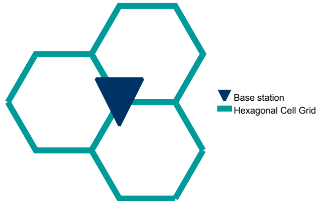
Figure 1 Hexagonal shaped mobile communication cell
