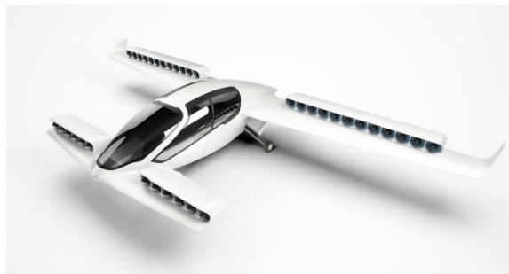
FIGURE 4.1.2-1: VECTORED THRUST VTOL
