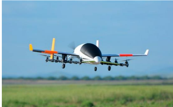
FIGURE 4.1.2-2: LIFT + CRUISE VTOL
