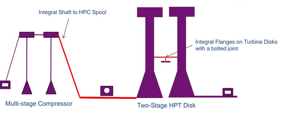
Example 4 – Two-Stage Turbine with Tie-bolt
