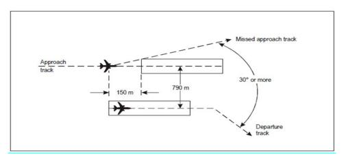
Figure 58: Segregated parallel operations where runways are staggered
