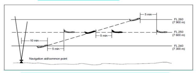
Figure 16: 5-minute separation between aircraft climbing and on the same track
