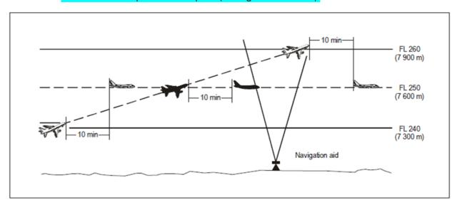
Figure 20: 10-minute separation between aircraft climbing and on crossing tracks
