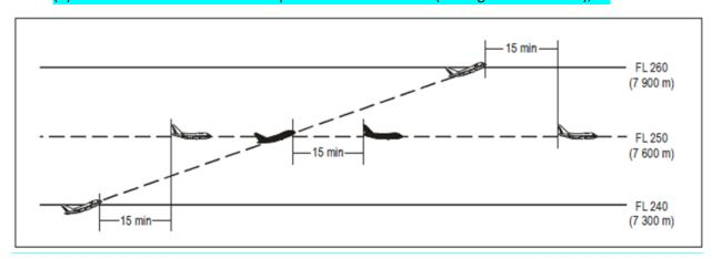
Figure 12: 15-minute separation between aircraft climbing and on the same track
