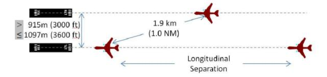
Figure 55: Diagonal separation for distance between centre lines greater than 915 m (3 000 ft) but less than or equal to 1 097 m (3 600 ft)
