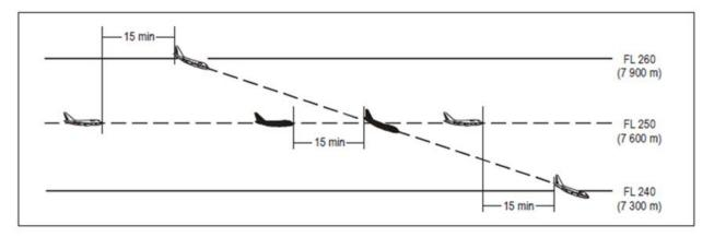
Figure 13: 15-minute separation between aircraft descending and on the same track
