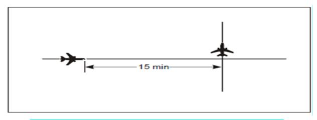
Figure 10: 15-minute separation between aircraft on crossing tracks and same level
