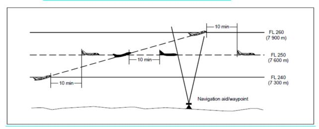
Figure 14: 10-minute separation between aircraft climbing and on the same track
