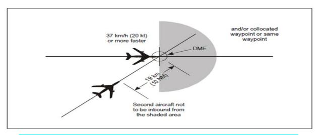
Figure 26: 19 km (10 NM) DME and/or GNSS-based separation between aircraft on crossing tracks and the same level
