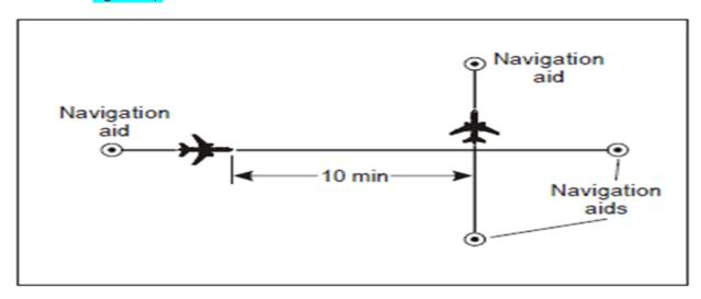
Figure 11: 10-minute separation between aircraft on crossing tracks and same level
