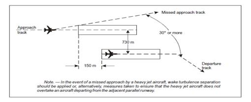
Figure 57: Segregated parallel operations where runways are staggered
