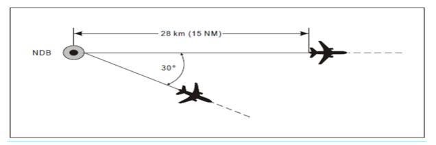
Figure 40: Separation using the same NDB
