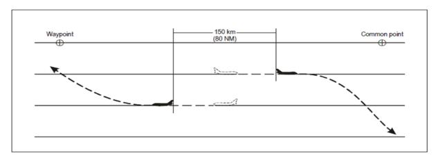
Figure 32: 150 km (80 NM) RNAV-based separation between aircraft on reciprocal tracks
