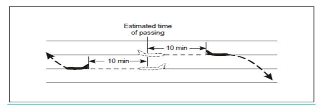
Figure 22: 10-minute separation between aircraft on reciprocal tracks
