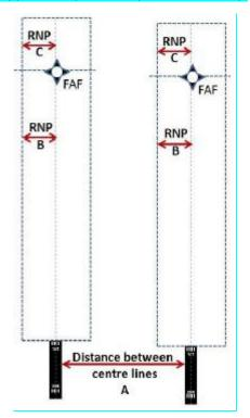
Figure 52: RNP value and distance between centre lines
