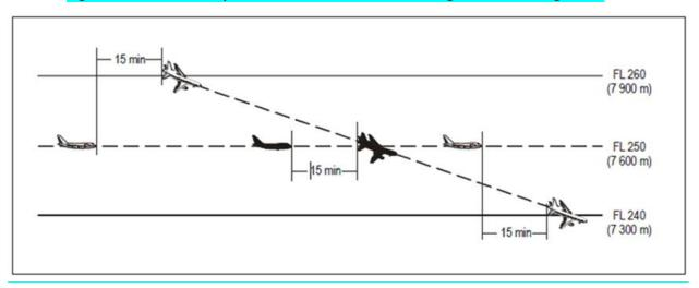
Figure 19: 15-minute separation between aircraft descending and on crossing tracks
