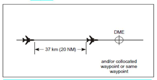
Figure 23: 37 km (20 NM) DME and/or GNSS-based separation between aircraft on the same track and same level
