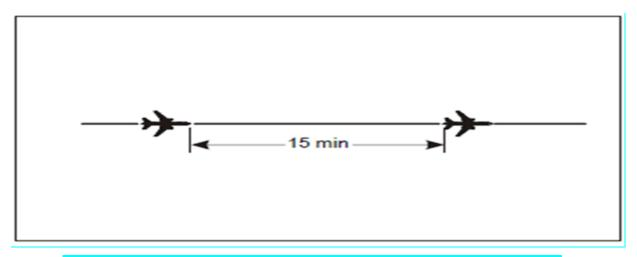
Figure 6: 15-minute separation between aircraft on the same track and same level
