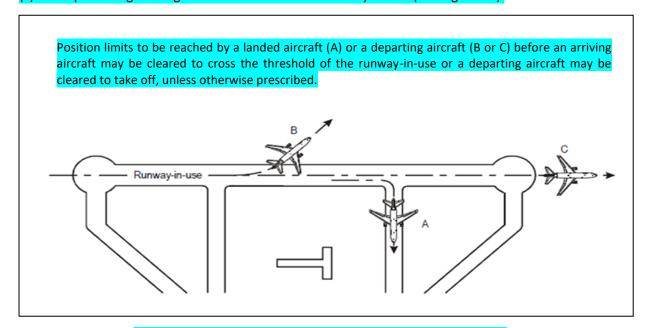
Figure 33: Separation between departing and arriving aircraft
