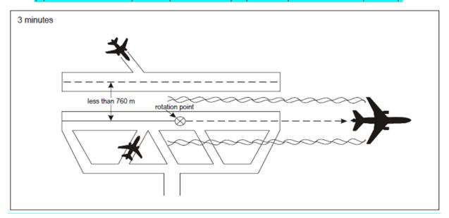
Figure 45: 3-minute wake turbulence separation for following aircraft
