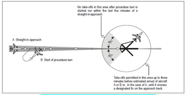
Figure 37: Separation of departing aircraft from arriving aircraft
