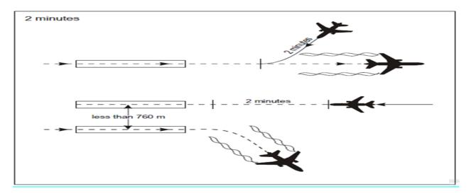
Figure 47: 2-minute wake turbulence separation for opposite-direction landing
