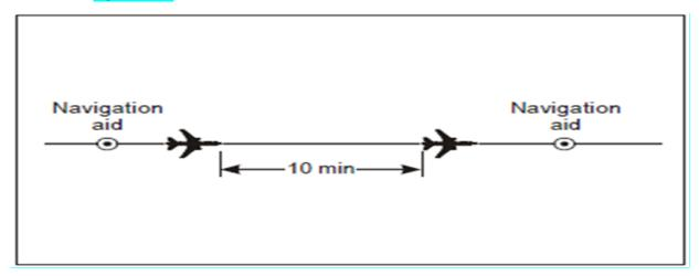
Figure 7: 10-minute separation between aircraft on the same track and same level
