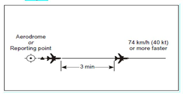
Figure 9: 3-minute separation between aircraft on the same track and same level
