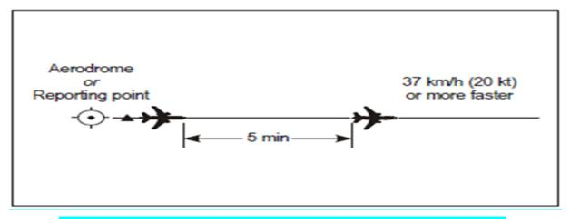
Figure 8: 5-minute separation between aircraft on the same track and same level
