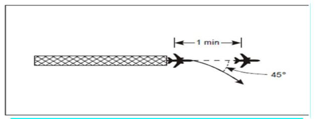
Figure 34: 1-minute separation between departing aircraft following tracks diverging by at least 45 degrees
