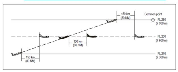
Figure 30: 150 km (80 NM) RNAV-based separation between aircraft climbing and on the same track
