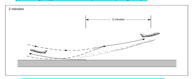
Figure 46: 2-minute wake turbulence separation for opposite-direction take-off
