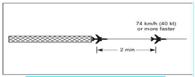
Figure 35: 2-minute separation between aircraft following the same track
