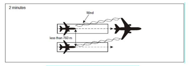
Figure 43: 2-minute separation for following aircraft
