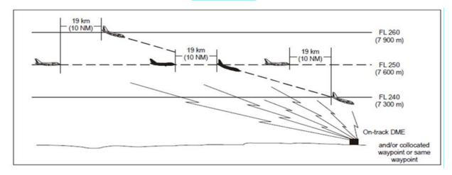
Figure 28: 19 km (10 NM) DME and/or GNSS-based separation between aircraft descending and on the same track
