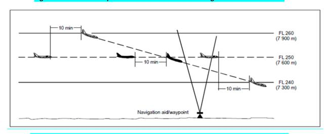
Figure 15: 10-minute separation between aircraft descending and on the same track
