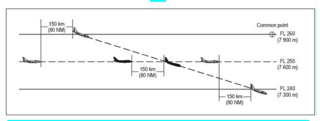
Figure 31: 150 km (80 NM) RNAV-based separation between aircraft descending and on the same track
