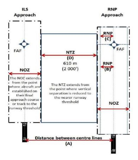
Figure 51: Distance between centre lines, NTZ and NOZ
