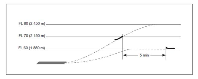
Figure 36: 5-minute separation of departing aircraft following the same track
