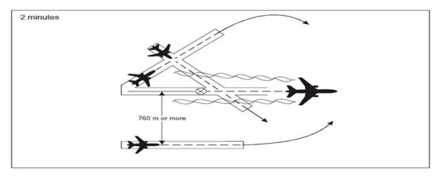
Figure 44: 2-minute wake turbulence separation for crossing aircraft
