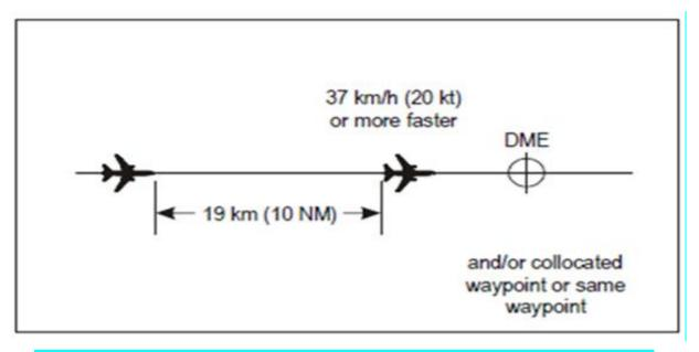
Figure 24: 19 km (10 NM) DME and/or GNSS-based separation between aircraft on the same track and same level
