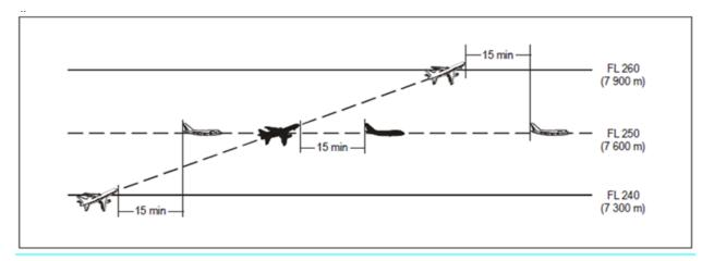
Figure 18: 15-minute separation between aircraft climbing and on crossing tracks
