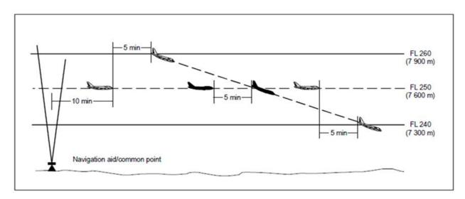
Figure 17: 5-minute separation between aircraft descending and on the same track
