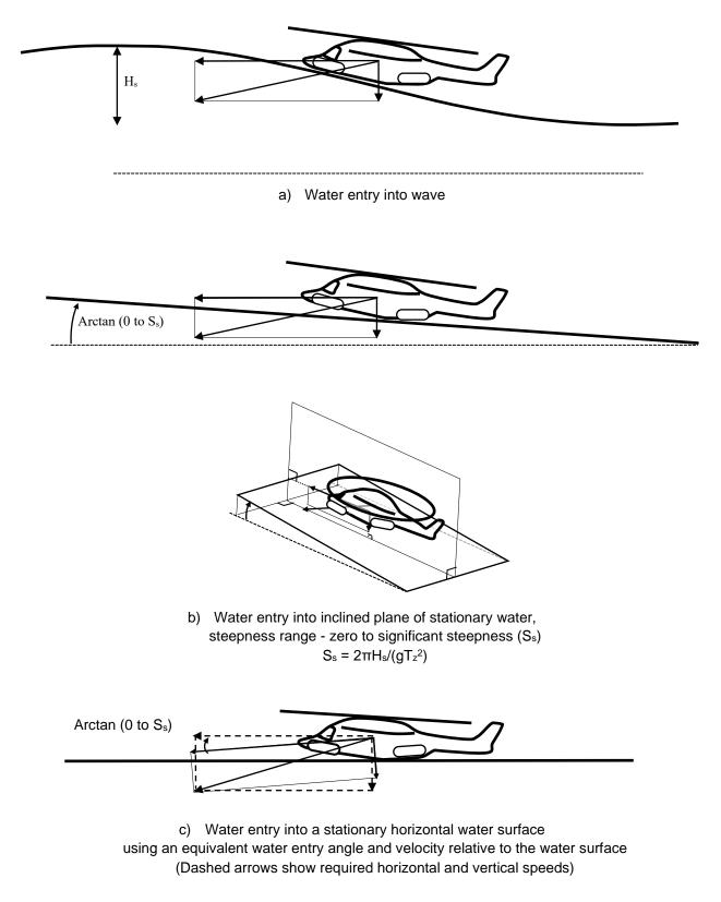
Figure 1 – Illustration of water entry test or simulation conditions which may be considered for structural provisions assessment
