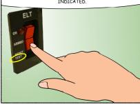
BEFORE DISPOSING OF THESE DEVICES, THEY SHOULD BE DISARMED AND THE BATTERIES REMOVED.
