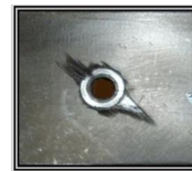
Hole delamination
