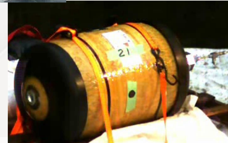
High strain impact (gunfire) test (SAE J2579)
