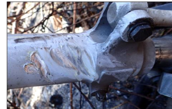
Figure 7: Impact damage to the pitch control mechanism
