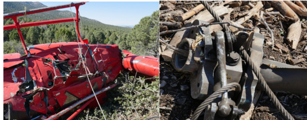
Figure 7: Impact damage to the pitch control mechanism
