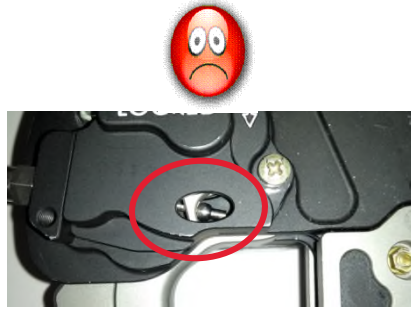
No Play between Ground Release Lever and Bowden Cable End
