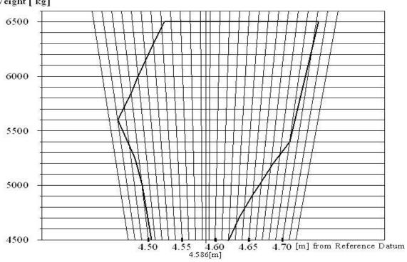
15. Datum: 2.470 m (97.24 in) Frame No. 9, Forward (see fig. 6.1, AFM, Chapter 6)
