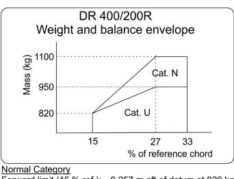
Forward limit (15 % ref.): .. 0.257 m aft of datum at 820 kg Intermediate limit (27 % ref.):0.462 m aft of datum at 1100 kg
