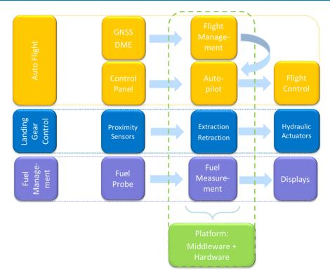
Figure 3 — Illustration of an IMA architecture
