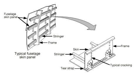
MED—the cracking of frames at stringer cutouts at successive longitudinal locations in the fuselage. The primary concern is for those areas where noncircular frames exist in the fuselage structure. Fractures in those areas would result in panel instability.
