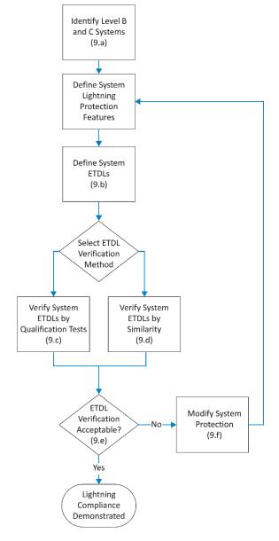
Figure 3 — Typical compliance process for Level B and C systems
