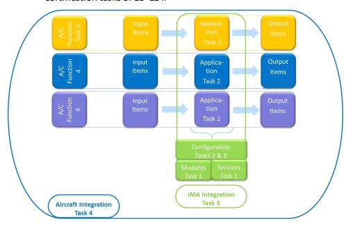
Figure 4 — Mapping between an IMA system and the ED-124 certification tasks
