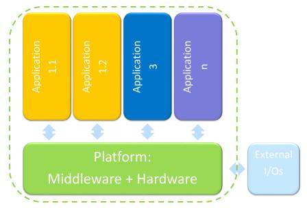
Figure 1 — Illustration of an IMA architecture
