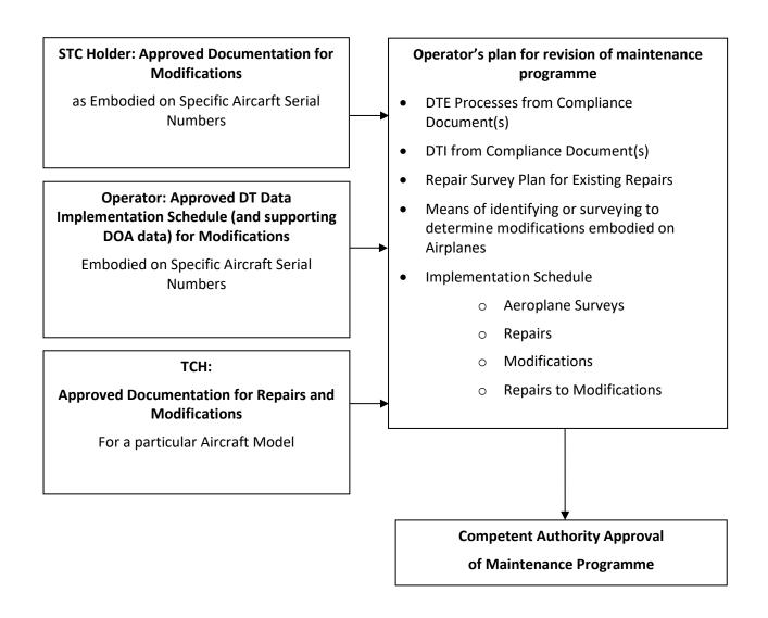
Figure A3-2 - Operator's Maintenance Programme Approval Process
