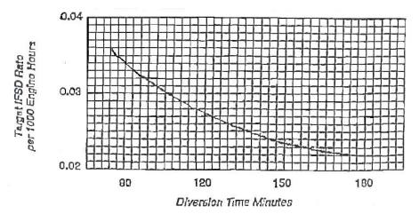
Figure 1: Target IFSD Rate versus Diversion Time
