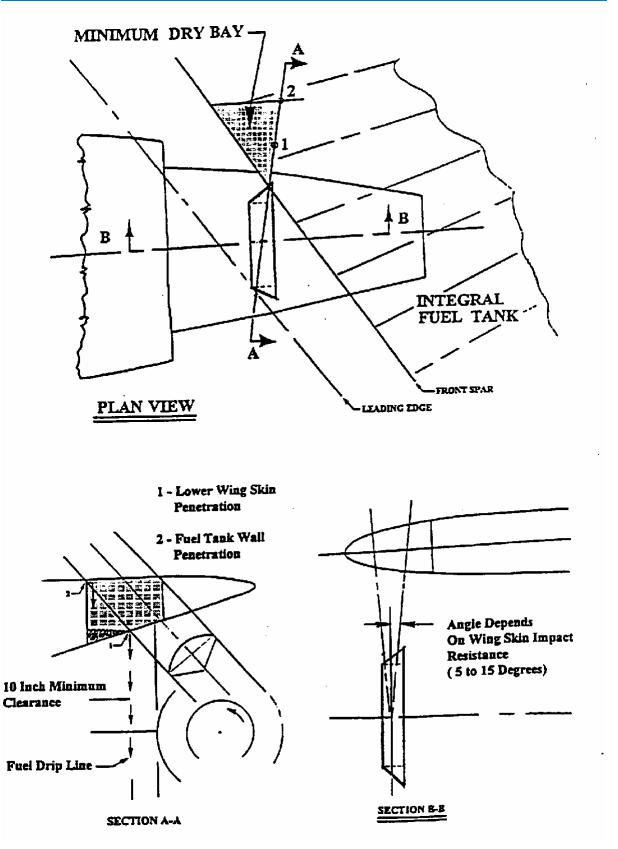
FIGURE 2 – DRY BAY SIZING DETERMINATION EXAMPLE
