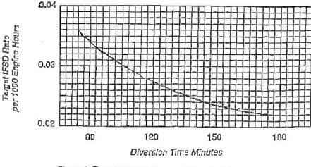
Figure 1: Target IFSD Rate versus Diversion Time
