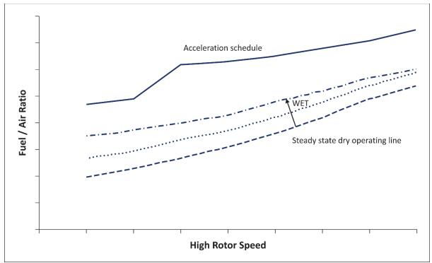
Figure 3 Typical Engine Control Characteristics
