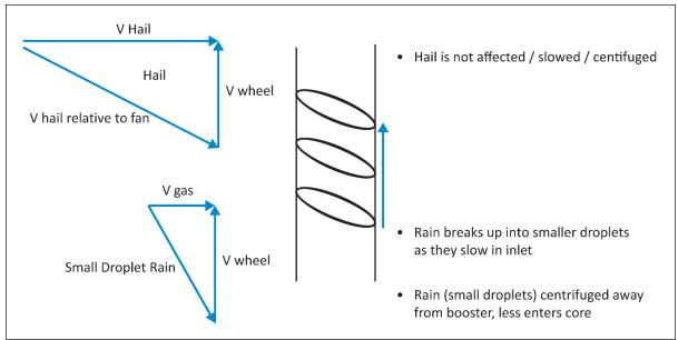
Figure 2 Velocity Vector Diagram
