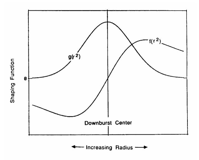
Figure 4 Characteristic Variation of Horizontal Shaping Functions
