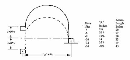
Assembly Flex Test Setup Figure III
