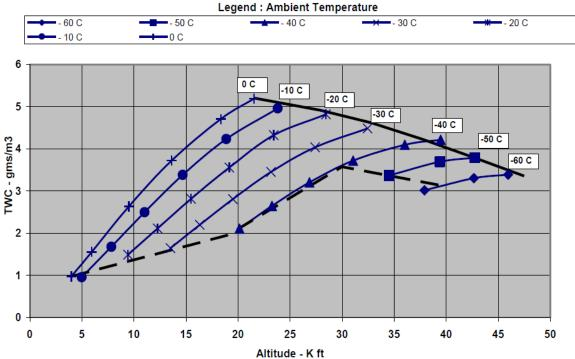
Ice crystal size median mass dimension (MMD) range is 50–200 microns (equivalent spherical size) based upon measurements near convective storm cores. The TWC can be treated as completely glaciated (ice crystal) except as noted in the Table 1.
