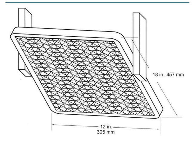
Figure 3b – Air Propane Radiant Panel
