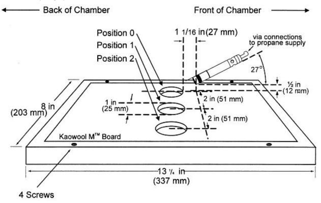
Figure 7 - Calorimeter Holding Frame
