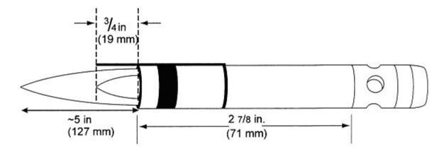
Figure 6 - Propane Pilot Burner
