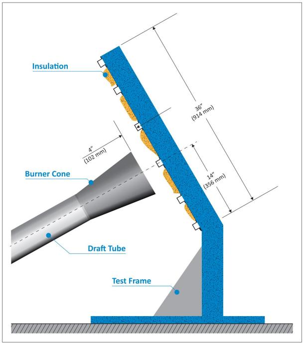
Figure 2 – Burnthrough Test Apparatus
