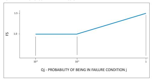
Figure 3: Factor of safety for continuation of flight
