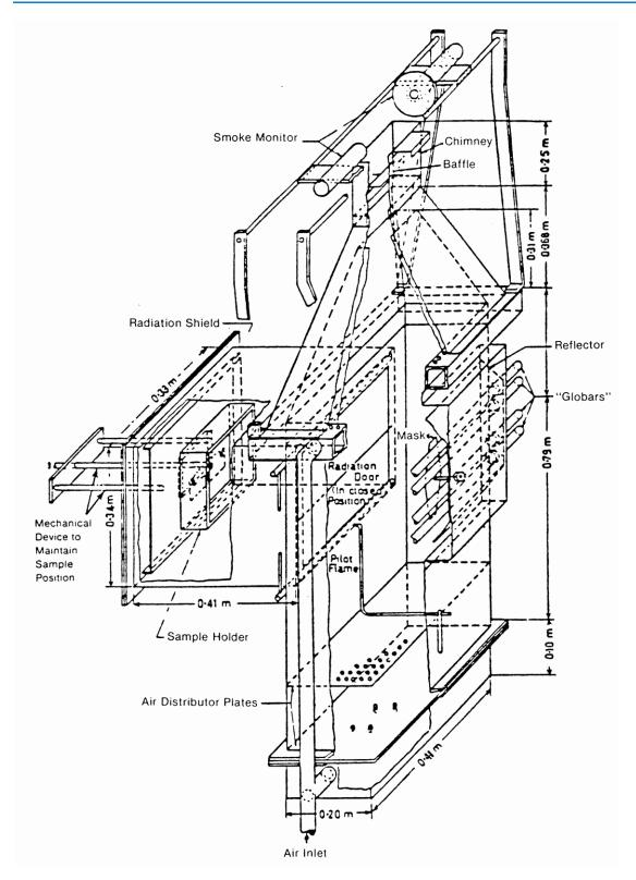
FIGURE 1. RELEASE RATE APPARATUS
