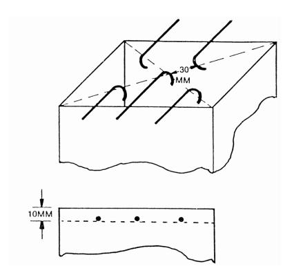
FIGURE 5. THERMOCOUPLE POSITION
