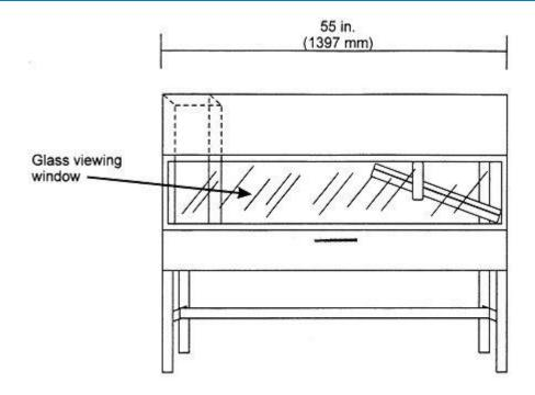
Figure 1 - Radiant Panel Test Chamber
