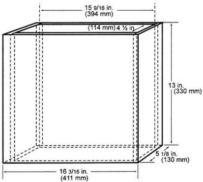
Figure 2 - Internal Chimney
