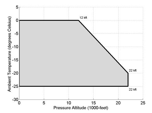
Figure 3 – Appendix O, Freezing Drizzle, Altitude and Temperature
