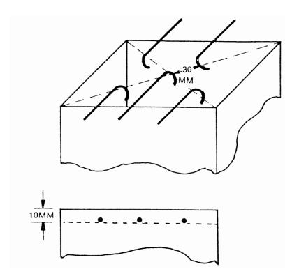
FIGURE 5. THERMOCOUPLE POSITION
