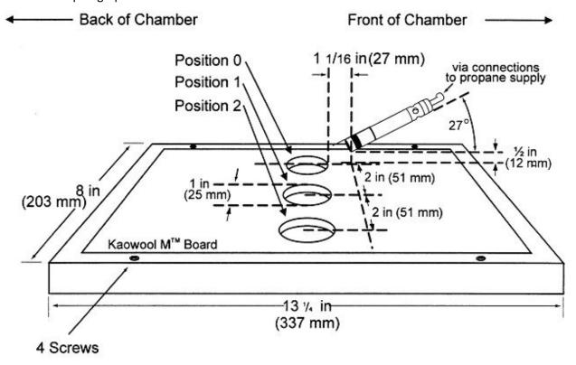
Figure 7 - Calorimeter Holding Frame
