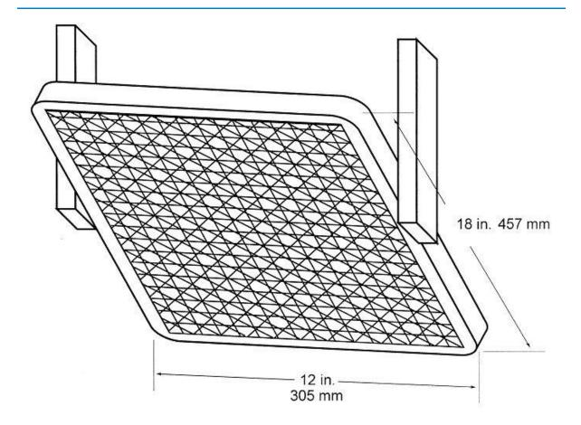
Figure 3b – Air Propane Radiant Panel
