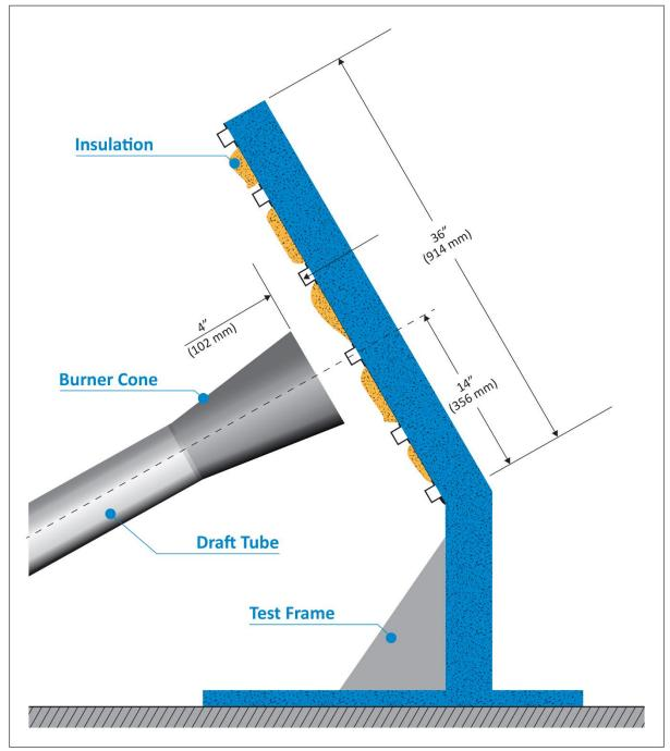
Figure 2 – Burnthrough Test Apparatus
