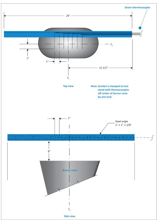
FIGURE 3 THERMOCOUPLE RAKE BRACKET
