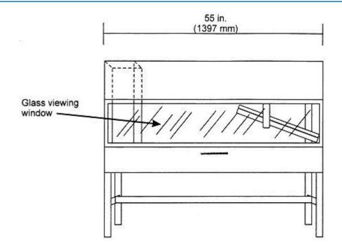
Figure 1 - Radiant Panel Test Chamber
