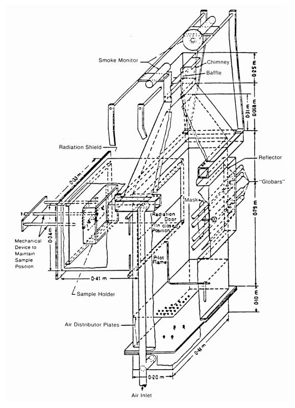
FIGURE 1. RELEASE RATE APPARATUS
