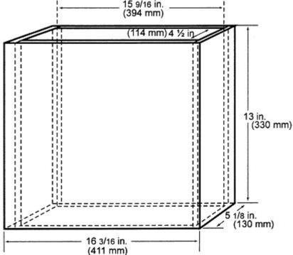
Figure 2 - Internal Chimney
