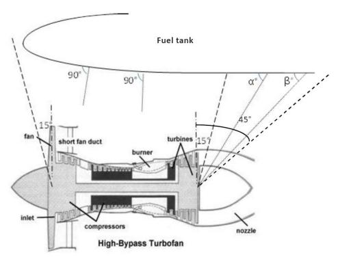
Note:  $\alpha$  and  $\beta$  angles are examples of possible angles between the fuel tank skin and the debris trajectory at the impact.
