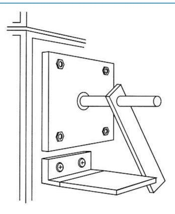
Figure 8 - Propane Burner Stop
