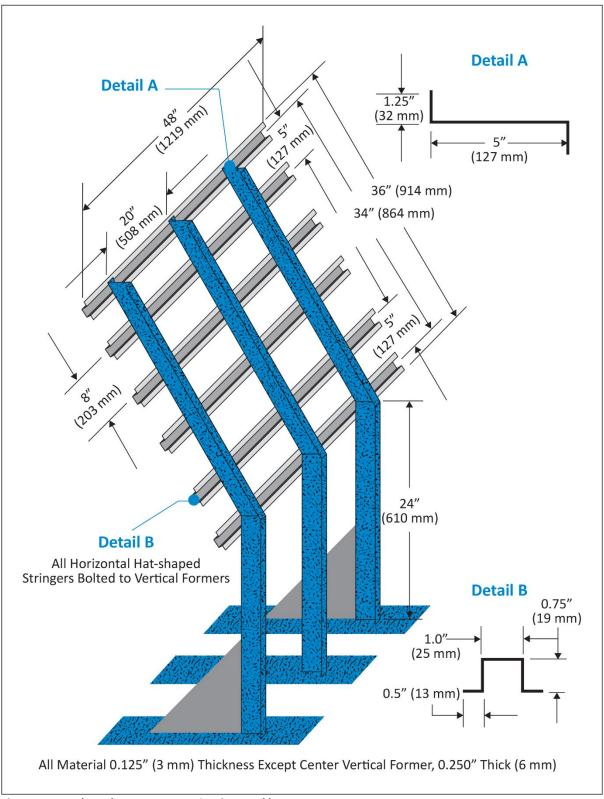
Figure 1 – Burnthrough Test Apparatus Specimen Holder
