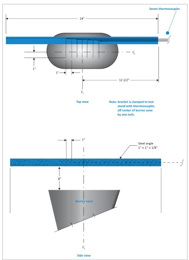
FIGURE 3 THERMOCOUPLE RAKE BRACKET
