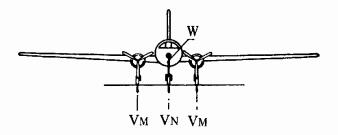
FIGURE 8 PIVOTING, NOSE- OR TAIL-WHEEL TYPE
