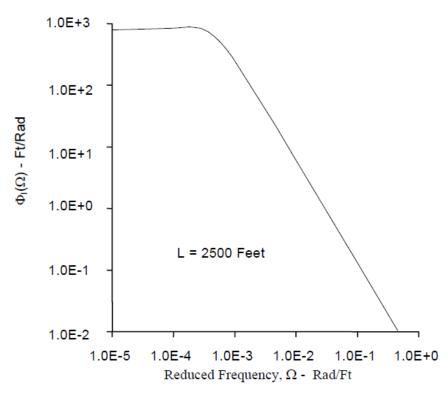
Figure-3 The Von Kármán Power Spectral Density Function,  $\Phi_i(\Omega)$
