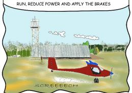
DURING THE INITIAL CLIMB, YOU HAVE VERY LITTLE TIME! IMMEDIATELY REDUCE THE ANGLE OF ATTACK BY PUSHING THE STICK FORWARD, GO STRAIGHT AHEAD MAINTAINING SPEED AND TRYING TO AVOID OBSTACLES IF POSSIBLE, USE THE REMAINING PART OF THE RUNWAY
