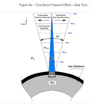
Figure 4c – Tyre Burst Pressure Effect – Bias Tyre Air jet pressure distribution
