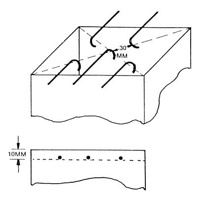
FIGURE 5. THERMOCOUPLE POSITION
