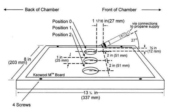
Figure 7 - Calorimeter Holding Frame
