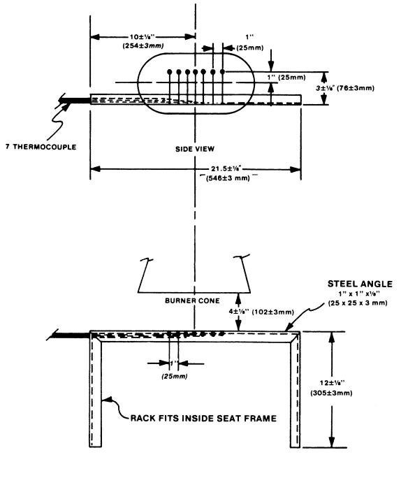
TOP VIEW THERMOCOUPLE RAKE BRACKET
