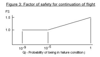
Qj = is the probability of being in the configuration with the unwanted in-flight thrust reversal
