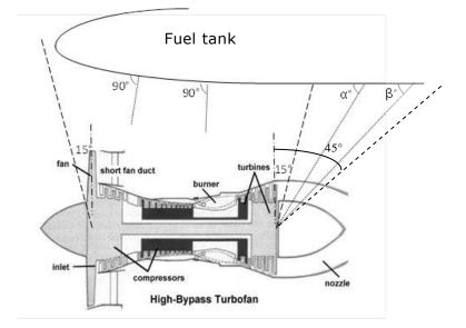
Note:  $\alpha$  and  $\beta$  angles are examples of possible angles between the fuel tank skin and the debris trajectory at the impact.
