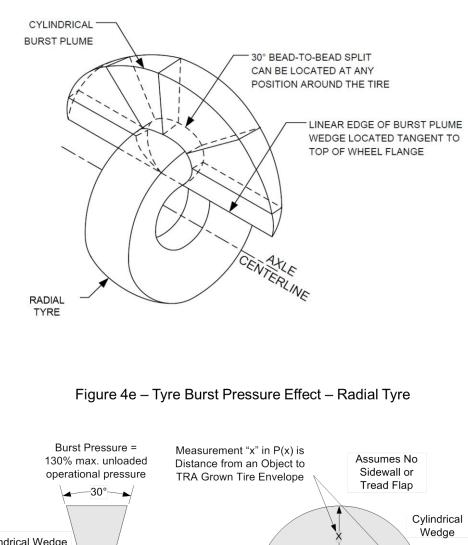
Figure 4d – Tyre Burst Pressure Effect – Radial Tyre
