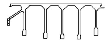
4.b - Deep Bore Disk Drum Rotor Cross Section
