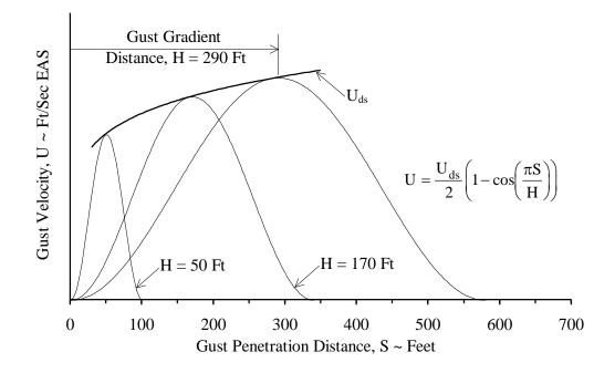
Figure-2 Typical (1-cosine) Design Gust Velocity Profiles
