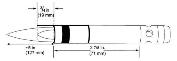
Figure 6 - Propane Pilot Burner
