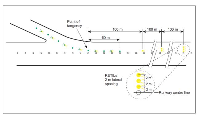
(5) Rapid exit taxiway indicator lights chromaticity should be in accordance with the specifications in CS ADR-DSN.U.930 and Figure U-1.
