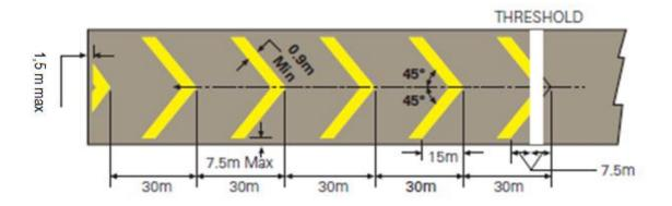
Figure R-2. Pre-threshold area marking
