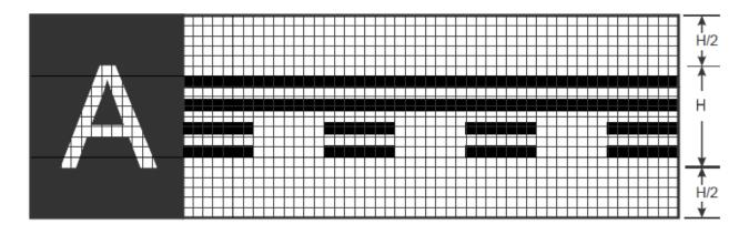
Figure N-2F- Runway vacated sign with typical location sign
