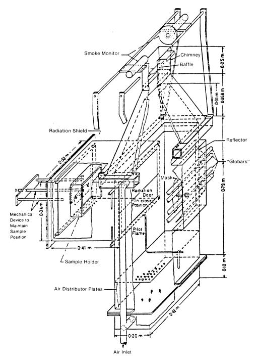
FIGURE 1. RELEASE RATE APPARATUS
