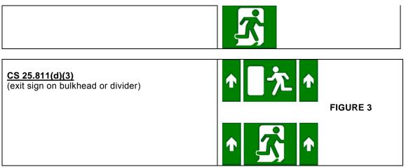
The design of symbolic exit signs should be chosen to provide a consistent set throughout the cabin.
