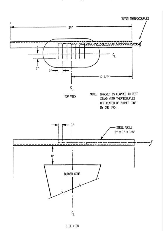
FIGURE 3 THERMOCOUPLE RAKE BRACKET
