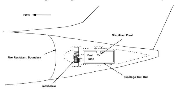
Figure 3- Example of Distances For Fuel Forward Acting
