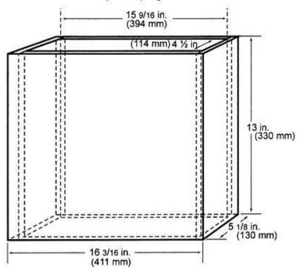
Figure 2 - Internal Chimney
