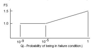
Qj = is the probability of being in the configuration with the unwanted in-flight thrust reversal
