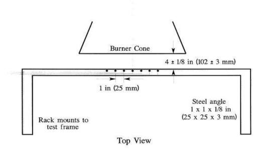
Figure 5 - Thermocouple Rake Position Relative to Burner Cone
