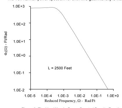
Figure-3 The Von Kármán Power Spectral Density Function,  $\Phi_{\underline{I}}(\Omega)$
