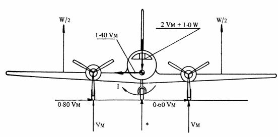
VM = One-half the maximum vertical ground reaction obtained at each main gear in the level landing conditions.
