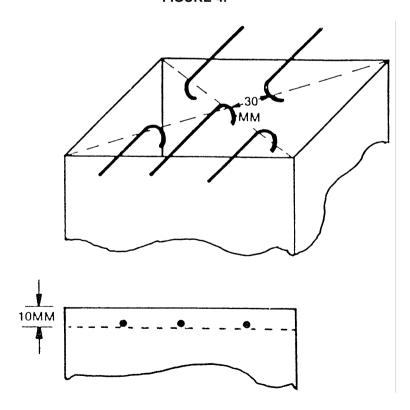
FIGURE 5. THERMOCOUPLE POSITION
