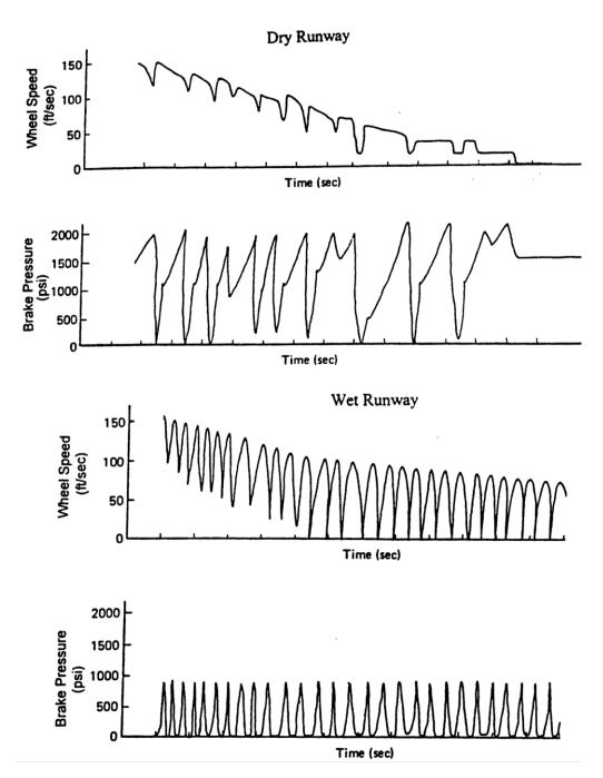
FIGURE 2. ANTI-SKID SYSTEM RESPONSE CHARACTERISTICS
