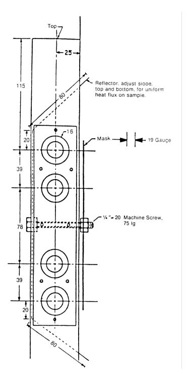
FIGURE 2B. "GLOBAR" RADIANT PANEL
