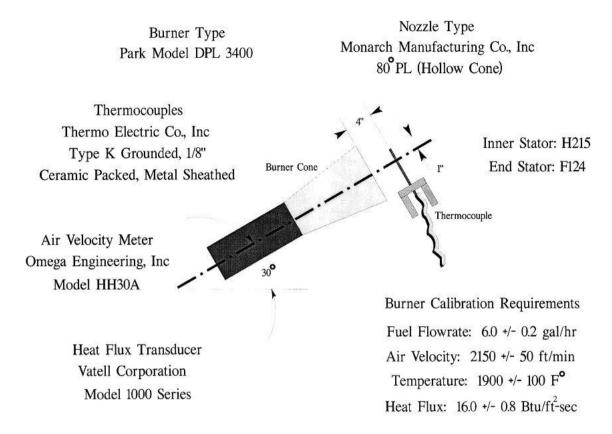
Figure 8 – Burner Information and Calibration Settings
