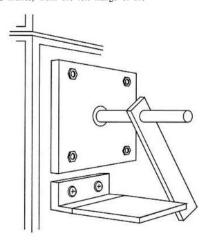
Figure 8 - Propane Burner Stop
