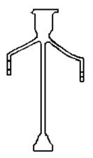
4.c - Single Stage Deep Bore Disk Cross Section
