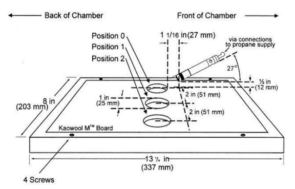
Figure 7 - Calorimeter Holding Frame
