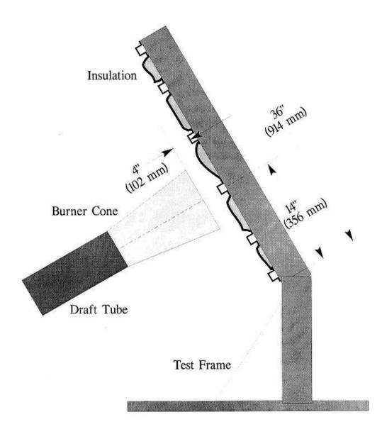
Figure 2 - Burnthrough Test Apparatus
