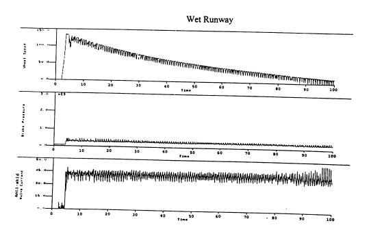
FIGURE 3. ANTI-SKID SYSTEM RESPONSE CHARACTERISTICS Fully Modulating System
