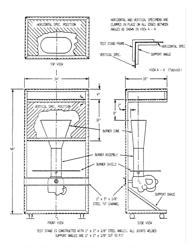
FIGURE 1 TEST APPARATUS FOR HORIZONTAL AND VERTICAL MOUNTING
