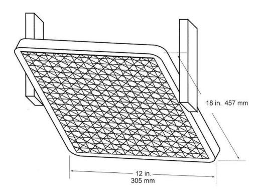
Figure 3b - Air Propane Radiant Panel
