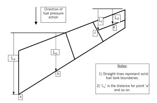
Figure 4 - Example of Distances For Fuel Outboard Acting
