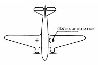
VN AND VM ARE STATIC GROUND REACTIONS. FOR TAIL-WHEEL TYPE THE AEROPLANE IS IN THE THREE POINT ATTITUDE. PIVOTING IS ASSESSED TO TAKE PLACE ABOUT ONE MAIN LANDING GEAR UNIT.
