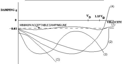
FIGURE 4: DAMPING VERSUS VELOCITY - Method 2
