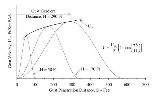
Figure-2 Typical (1-cosine) Design Gust Velocity Profiles
