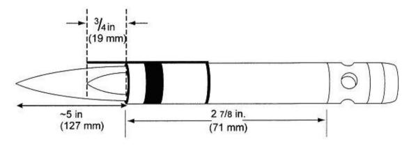
Figure 6 - Propane Pilot Burner
