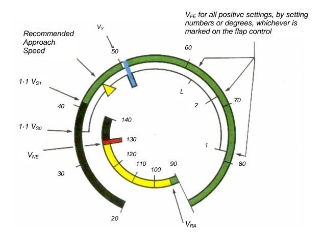
FIGURE 1 EXAMPLE OF AIR SPEED INDICATOR MARKINGS
