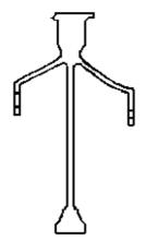
4.c - Single Stage Deep Bore Disk Cross Section
