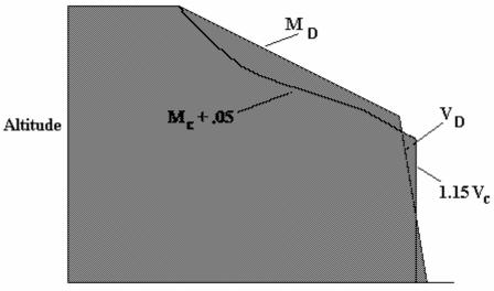
FIGURE 1B MINIMUM FAIL-SAFE CLEARANCE ENVELOPE
