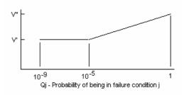
Figure 3: Clearance speed
