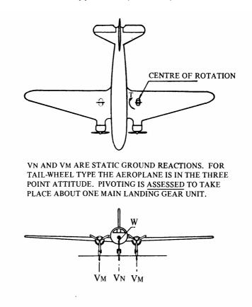
FIGURE 8 PIVOTING, NOSE- OR TAIL-WHEEL TYPE
