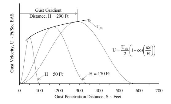
Figure-2 Typical (1-cosine) Design Gust Velocity Profiles
