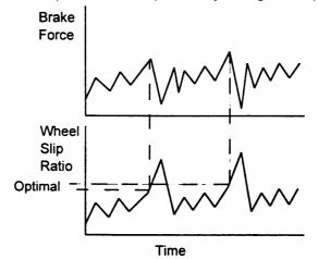
FIGURE 6. SUBSTANTIATION OF THE OPTIMAL SLIP VALUE
