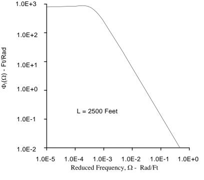
Figure-3 The Von Kármán Power Spectral Density Function, Φ<sub>l</sub>(Ω)
