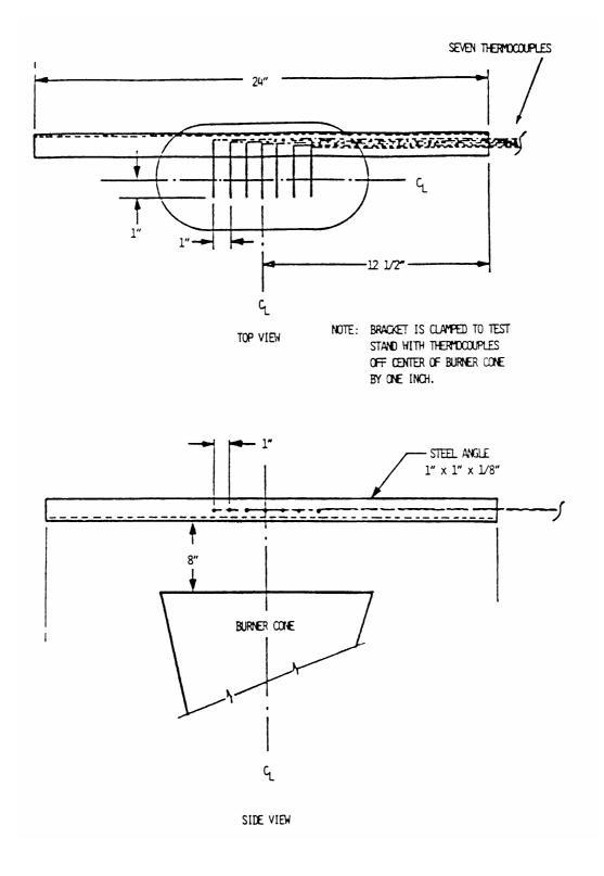
FIGURE 3 THERMOCOUPLE RAKE BRACKET
