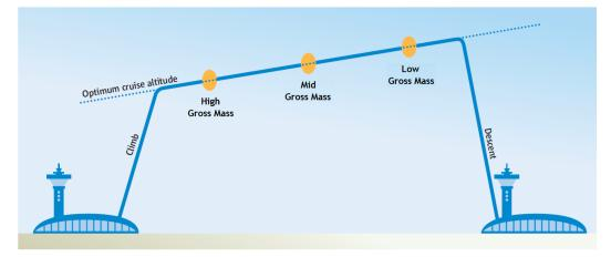
Figure 2 — Illustrative example of the three SAR measurement points for  $CO_2$  emission evaluation
