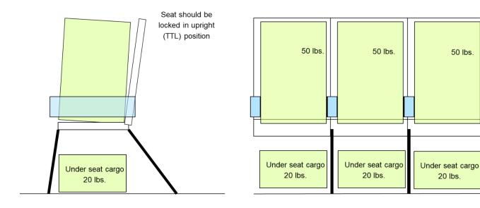
Interim cargo transportation on seat for 1 box maximum 50kg (110 lbs) Maximum height of cargo not higher than top of seat backrest Cargo restraint means are not shown.
