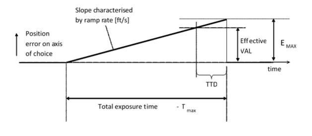
**Figure 7: Malfunction transient**
