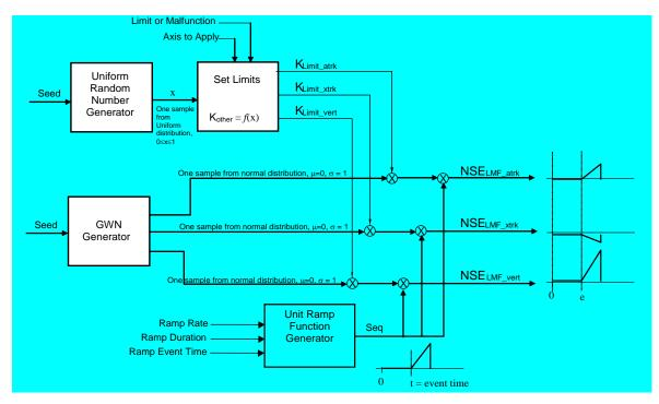
Figure 6: Limit malfunction generator
