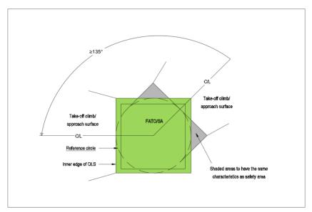
Figure D-2. Square FATO with reference circle and surfaces separated by 135°
