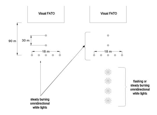
Figure E-18. Two different configurations of an approach lighting system
