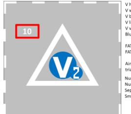
V height 260 cm V width 260 cm V base 70 cm V line width 60 cm V vertex height 90 cm Blue circle ∅ 340 cm
