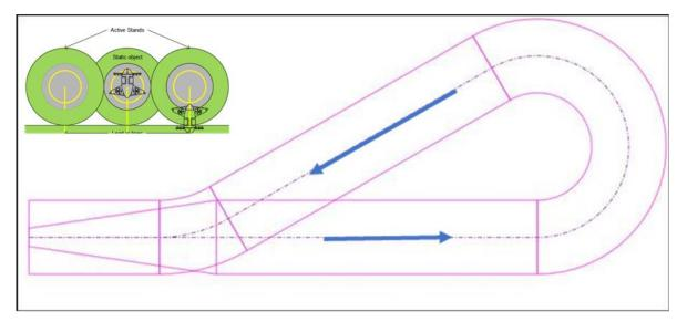
Figure C-6. Example of not providing parking stands under a flight path
