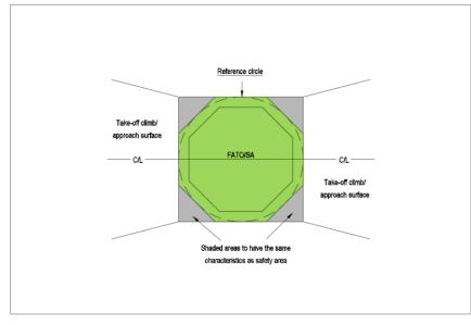
Figure D-3. Octagonal FATO with reference circle and diametrically opposed surfaces
