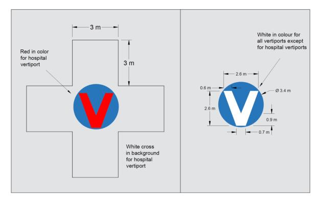
Figure E-4. Hospital vertiport identification and vertiport identification marking
