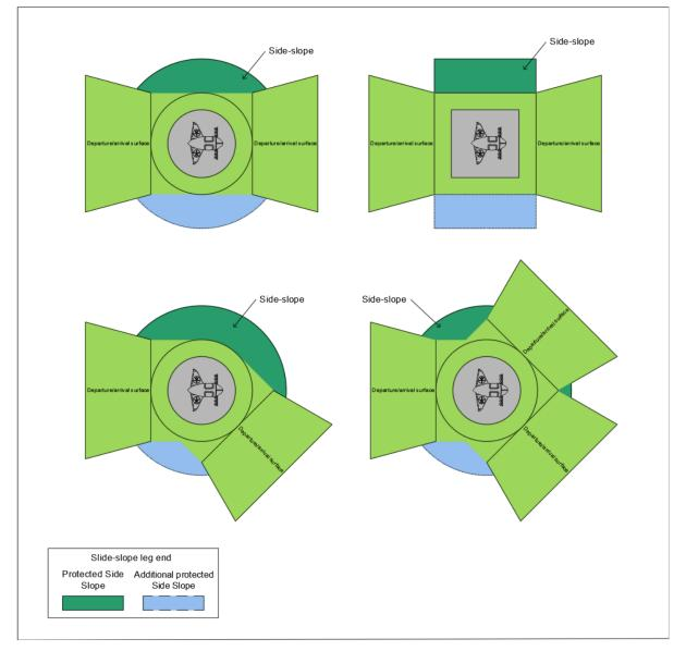
(b) The surface of a protected side slope should not be penetrated by obstacles.
