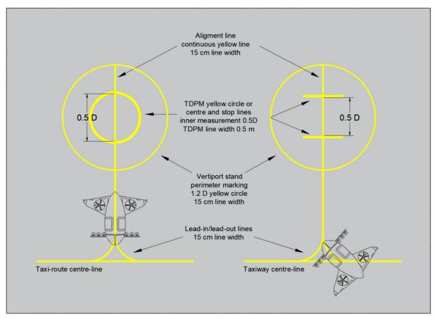
Figure E-13. VTOL-capable aircraft stand markings
