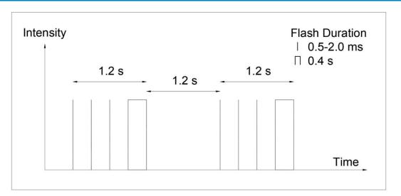
Figure E-16. Vertiport beacon flash characteristics
