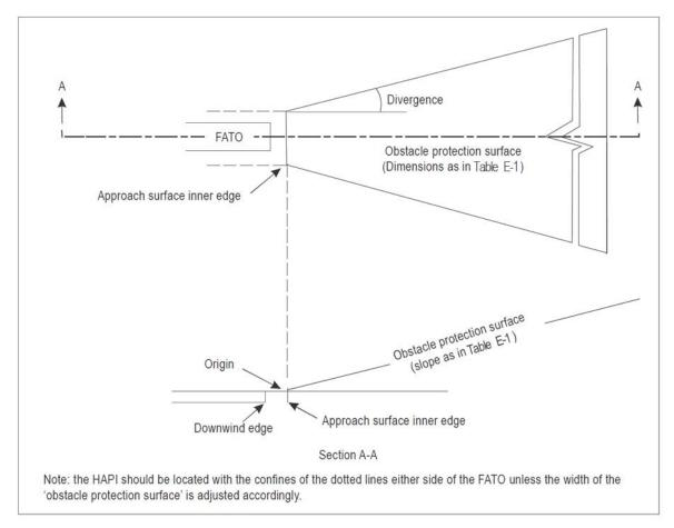
Figure E-24. Obstacle protection surface
