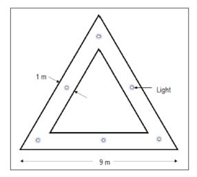
Figure E-8. Aiming point marking
