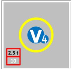
V height 260 cm V width 260 cm V base 70 cm V line width 60 cm V vertex height 90 cm Blue circle ∅ 340 cm
