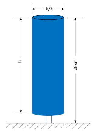
Figure E-10. VTOL-capable aircraft taxiway edge marker
