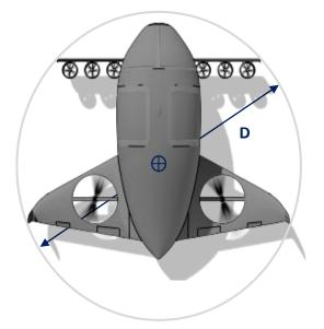
Figure D-23. Dimension 'D' and centre of the smallest enclosing circle
