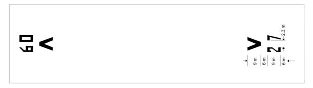
Figure E-3. FATO designation marking and vertiport identification marking for a runway-type FATO
