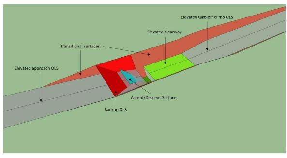
Figure D-11. Elevated OLS and transitional surface
