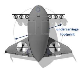
Figure D-26. Undercarriage footprint
