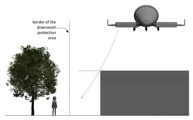
Figure C-2. Downwash protection area extended below the vertiport that is elevated
