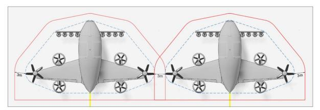
Figure C-8. VTOL-capable aircraft stands with a protection area
