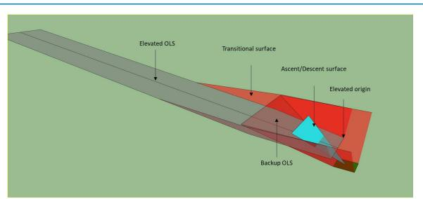
Figure D-8. Transitional, backup and approach surface
