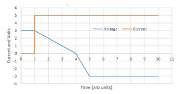
Figure 2-8: Typical Current / Voltage diagram vs time for a cell driven into polarity reversal. After the cell capacity is depleted to zero volts (time step 4) and the cell becomes resistive, the voltage across the cell will rapidly be driven negative by continued current from the power supply.
