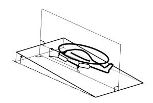
b) Water entry into inclined plane of stationary water, steepness range - zero to significant steepness ( $S_s$ )  $S_s = 2\pi H_s/(gT_z^2)$
