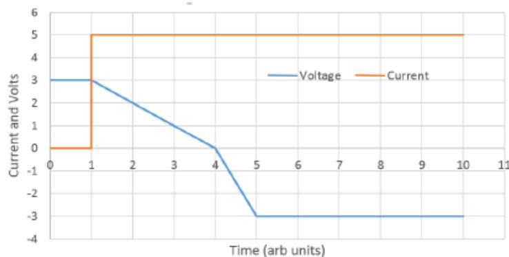
**Figure 2-8:** Typical Current / Voltage diagram vs time for a cell driven into polarity reversal. After the cell capacity is depleted to zero volts (time step 4) and the cell becomes resistive, the voltage across the cell will rapidly be driven negative by continued current from the power supply.
