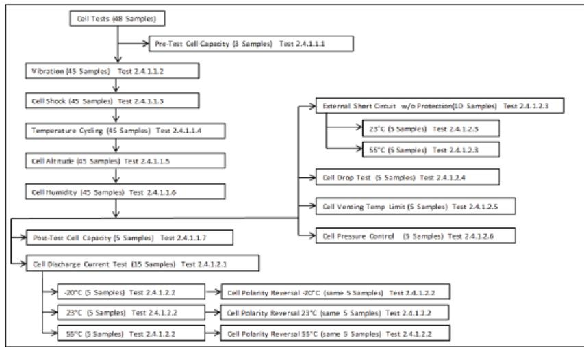
**Figure 2-25: Cell Test Sequence**
