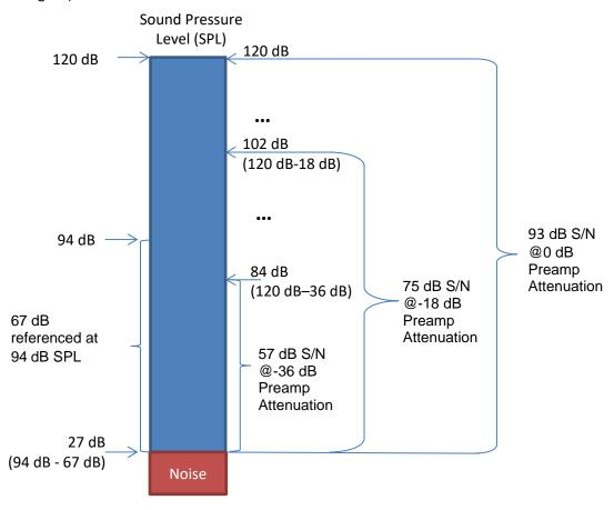
$$SPL_{maximum} = 120 \; dB - Selectable \; input \; attenuation$$
