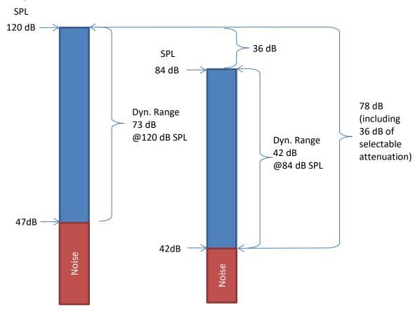
Dynamic Range is implicitly defined by the SNR Values 42 dB + 36 dB of selectable attenuation. This results in "78 dB including 36 dB of selectable attenuation".
