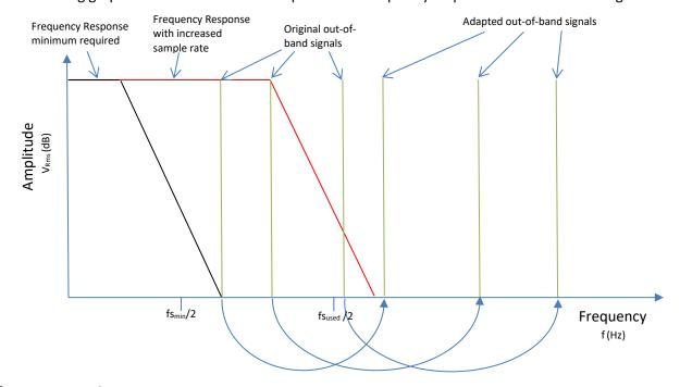
$fs_{min} = 11.025 \text{ kHz}$  $fs_{used} = 22.050 \text{ kHz}$
