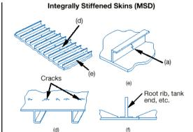
Do not have inherent crack stopper characteristics of riveted skin and stringer construction
