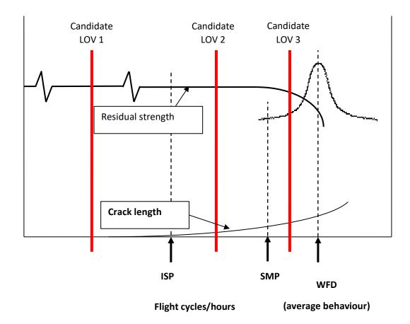
Figure 2-1: Comparison of WFD-susceptible structure to aircraft LOV
