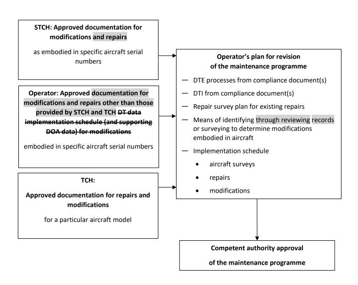
Figure A3-2: Operator's maintenance programme approval process
