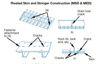
Inherent fail safe and crack stopper characteristics
