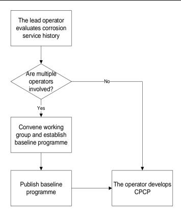
Figure A4-3: Operator-developed baseline CPCP
