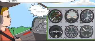
THE HORN STALL WARNING IS ADJUSTED TO START 5 TO 10 KT BEFORE THE STALL
