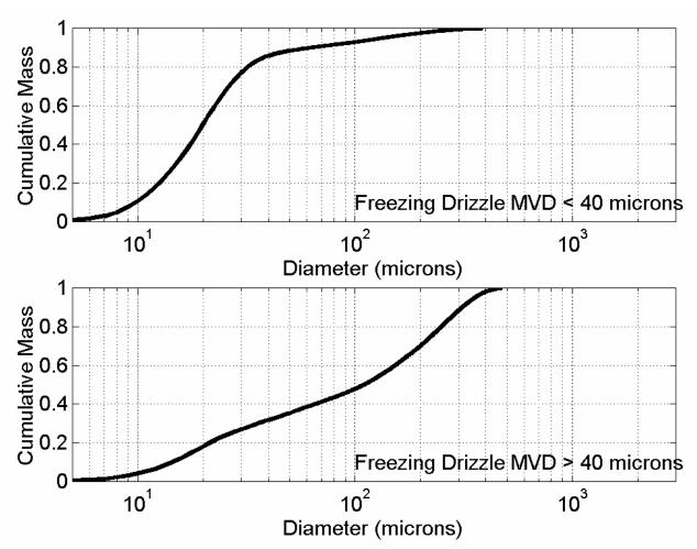
Figure 2 – Appendix O, Freezing Drizzle, Drop Diameter Distribution
