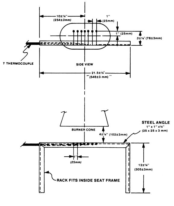
TOP VIEW THERMOCOUPLE RAKE BRACKET
