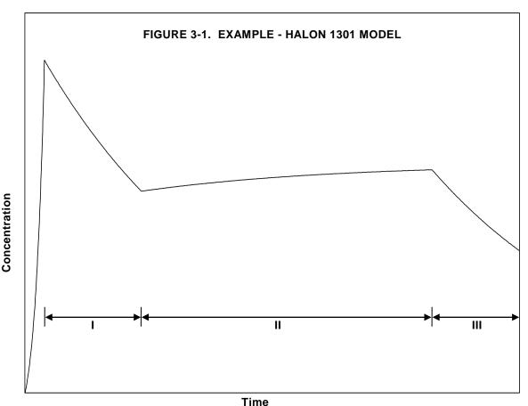
The second type of Halon 1301 discharge method slowly releases the fire-extinguishing agent from one or more pressurised bottles into the cargo compartment. This type of discharge method is commonly known as a metering system.
