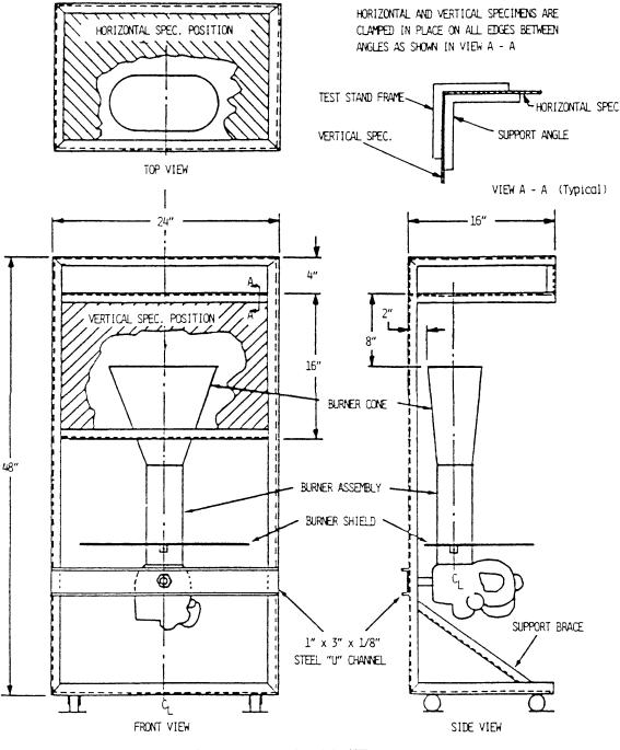
TEST STAND IS CONSTRUCTED WITH 1" x 1" x 1/8" STEEL ANGLES, ALL JOINTS WELDED SUPPORT ANGLES ARE 1" x 1" x 1/8" CUT TO FIT
