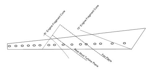
Figure 2 — Example of the  $\pm$  15-degree threat area representation Note: The threat area between - 15 and - 45 degrees is not represented.
