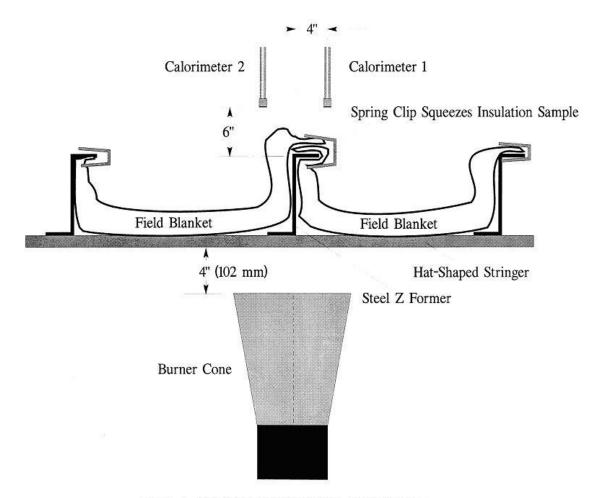
Figure 7 - Test Specimen Installation on Test Frame
