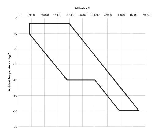
Within the envelope, total water content (TWC) in  $g/m^3$  has been determined based upon the adiabatic lapse defined by the convective rise of 90 % relative humidity air from sea level to higher altitudes and scaled by a factor of 0.65 to a standard cloud length of 32.2 km (17.4 nautical miles). Figure 2 displays TWC for this distance over a range of ambient temperature within the boundaries of the ice crystal envelope specified in Figure 1.
