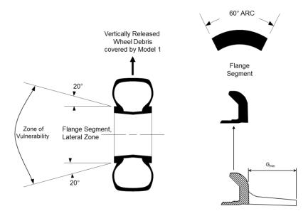
Figure 2 - Wheel Flange Release Threat
