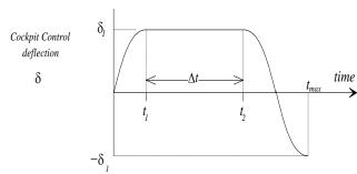
(iv) In cases where the cockpit pitch control motion may be affected by inputs from systems (for example, by a stick pusher that can operate at high load factor as well as at 1g) then the effects of those systems must be taken into account.
