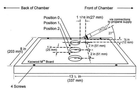
Figure 7 - Calorimeter Holding Frame
