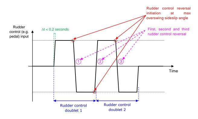
Figure 1: Illustration of the cockpit rudder control inputs
