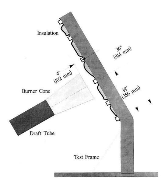
Figure 2 - Burnthrough Test Apparatus
