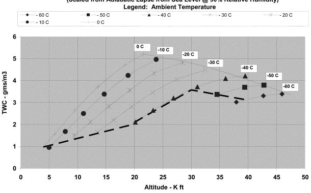
TWC Levels: Standard Exposure Length of 17.4 Nautical Miles (Scaled from Adiabatic Lapse from Sea Level @ 90% Relative Humidity)
