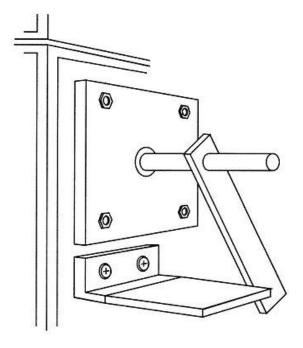
contact with the center of the specimen at the "zero" point and simultaneously start the timer. The pilot burner must be at a  $27^{\circ}$  angle with the sample and be approximately  $\frac{1}{2}$  inch (12 mm) above the sample. See figure 7. A stop, as shown in figure 8, allows the operator to position the burner correctly each time.
