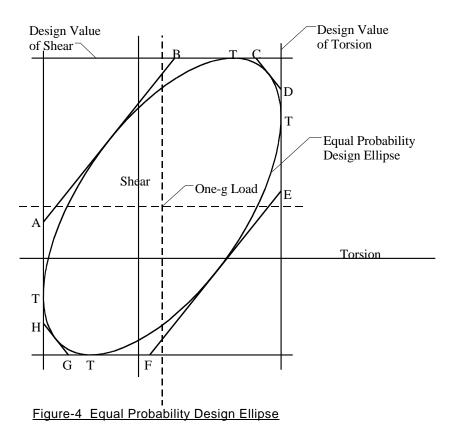
In this figure, the points of tangency, T, correspond to the expressions for correlated load pairs given by the foregoing expressions. A practical additional set of equiprobable load pairs that should be considered to establish critical design stresses are given by the points of tangency to the ellipse by lines AB, CD, EF and GH. These additional load pairs are given by the following expressions (where i = torsion and j = shear):
