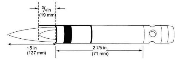
Figure 6 - Propane Pilot Burner
