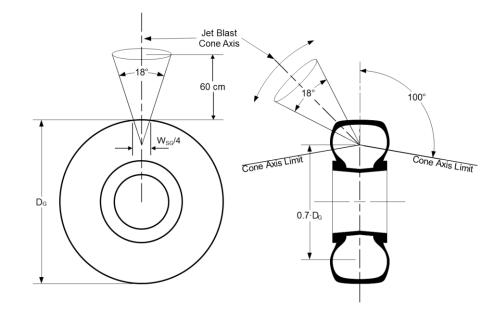
Figure 4a – Tyre Burst Pressure Effect – Bias Tyre
