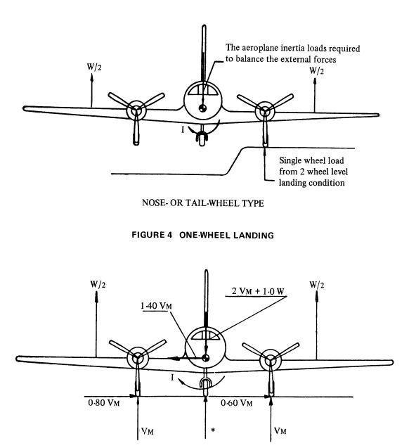
VM = One-half the maximum vertical ground reaction obtained at each main gear in the level landing conditions.
