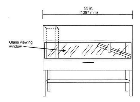
Figure 1 - Radiant Panel Test Chamber
