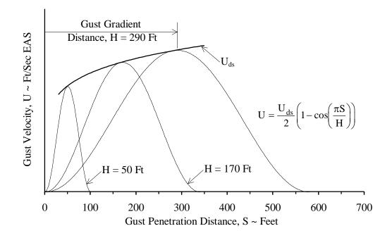
Figure-2 Typical (1-cosine) Design Gust Velocity Profiles
