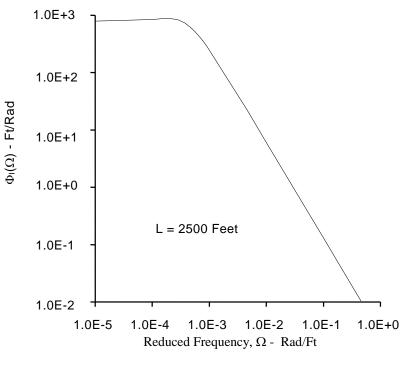
The Von Kármán power spectrum for unit RMS gust intensity is illustrated in Figure 3.
