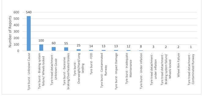
Figure 2: Overview of tyre and wheel failure reports
