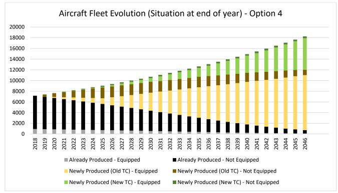
Figure 9 – Aeroplane Fleet Evolution for Option 4 (Equipped = either OBTPMS or GTPIS)
