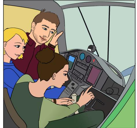
UN "GLASS COCKPIT", AVEC UN "PRIMARY FLIGHT DISPLAY" AND ET UN SECOND ÉCRAN MULTIFONCTIONNEL
