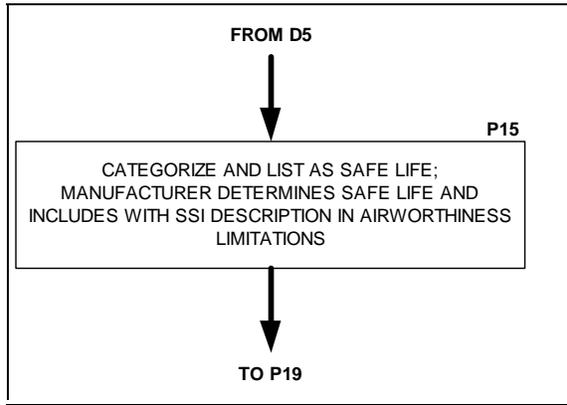
Figure 2-4-4.6. Fatigue Damage Analysis Logic Diagram
