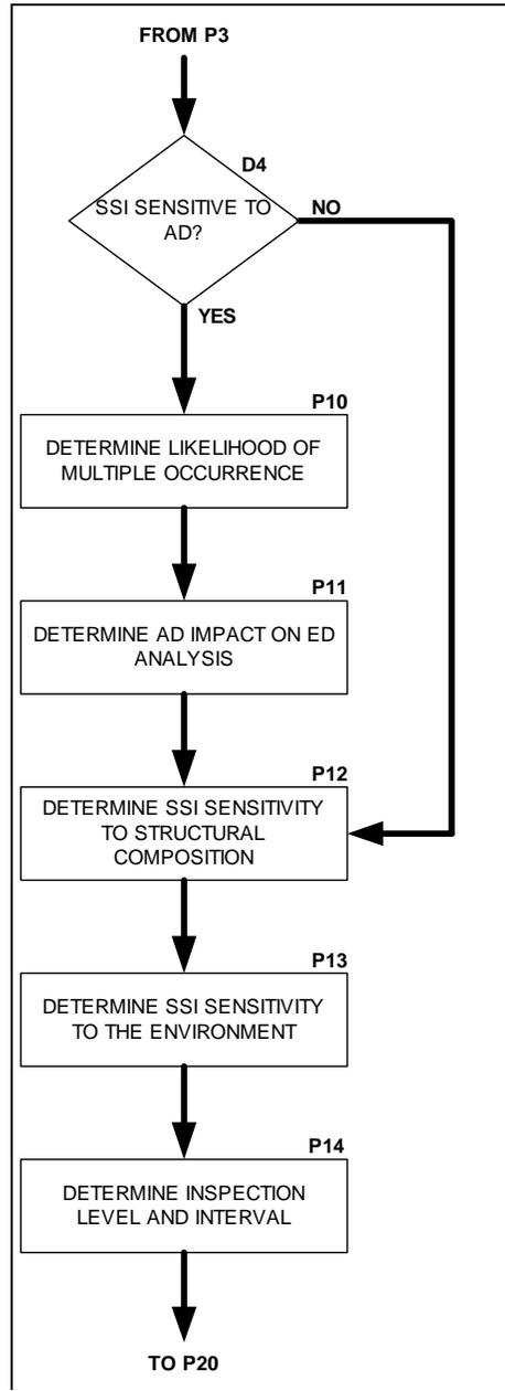
**Figure 2-4-4.5. Safelife Limit Analysis Logic Diagram**
