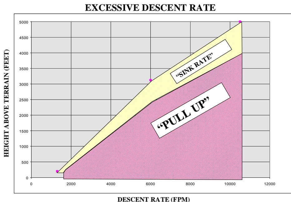
8.0 Class B Equipment Test Requirements for Negative Climb Rate or Altitude Loss After Takeoff. Use the existing performance envelopes specified in DO-161A based upon a „Height above Runway “ using barometric altitude (or equivalent) and runway elevation in lieu of radio altimeter inputs.
