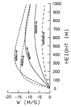
Figure 3 — Vertical Profile of Microburst Downflow
