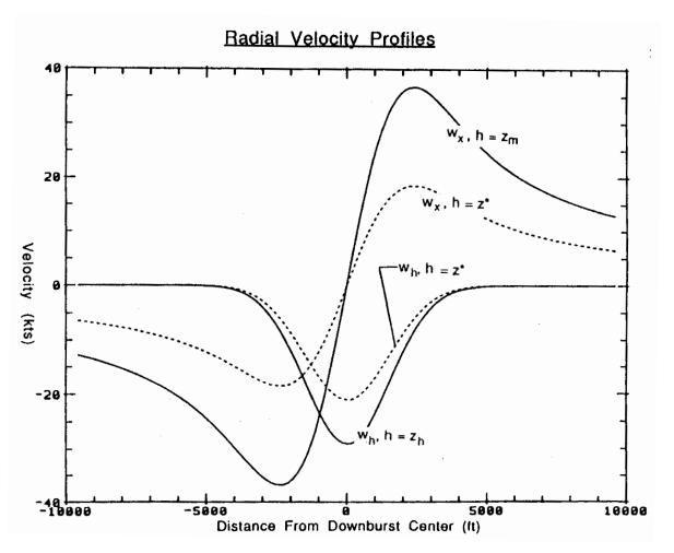
Figure 7 — Radial Velocity Profiles for the Analytical Model
