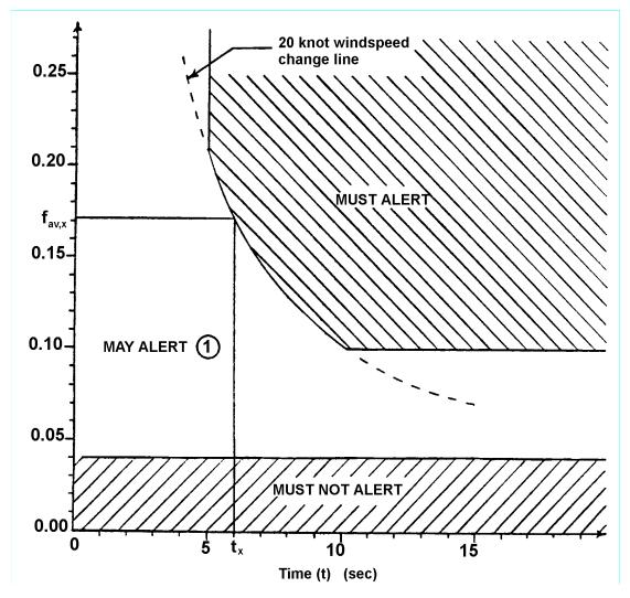
f<sub>av,x</sub> = average shear intensity to cause a warning at time t<sub>x</sub> (resulting in a 20-knot wind speed change, bounded as shown; applies to horizontal, vertical, and combination shear intensities),
