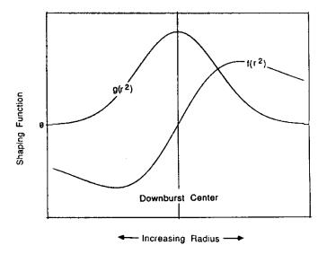
Figure 4 — Characteristic Variation of Horizontal Shaping Functions
