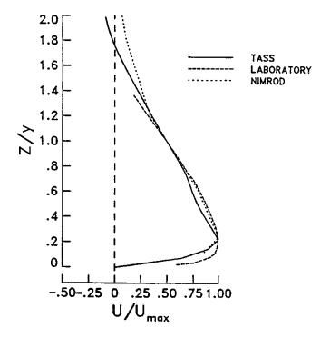
Figure 2 — Vertical Profile of Microburst Outflow (Non-dimensional)
