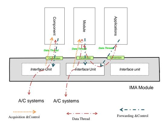
Figure 20: IMA module overview for ETSO-2C153 CLASS IF
