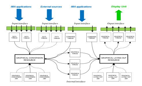
Figure 18: CLASS GP Graphical Processing (GP) elements relationship
