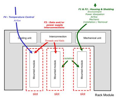
Figure 6: IMA module overview for ETSO-2C153 CLASS RH
