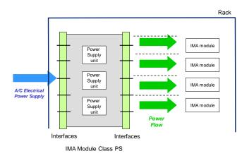
Figure 22: IMA module overview of ETSO-2C153 CLASS PS
