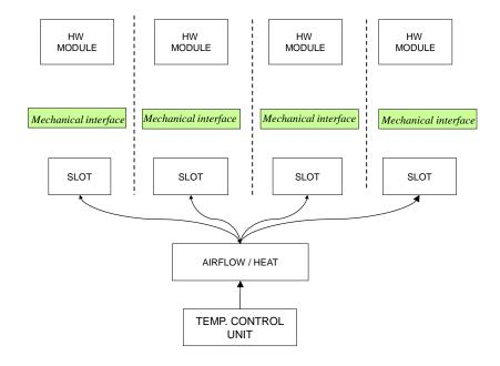
Figure 14: CLASS RH Cooling elements relationship
