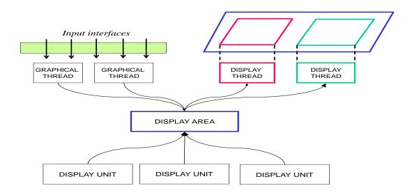
Figure 25: CLASS DH Display Head elements' relationship
