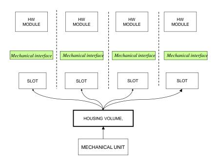
Figure 8: CLASS RH Housing elements relationship
