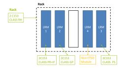
Figure 3 — IMA modules installed in a Rack Module
