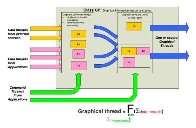
Figure 17: IMA module overview for ETSO-2C153 CLASS GP
