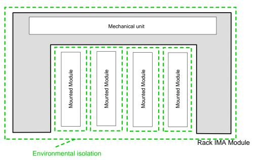
Figure 9: CLASS RH Shielding function overview
