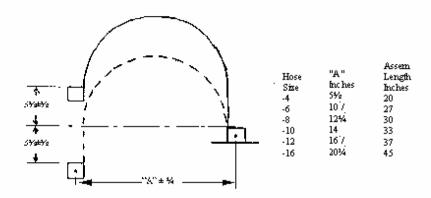
Assembly Flex Test Setup Figure III
