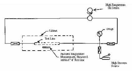
Typical Setup for High Temperature Pressure Testing Figure II
