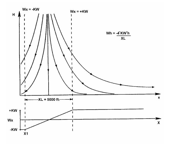
Figure 1 Wind Model Used In Guidance Studies
