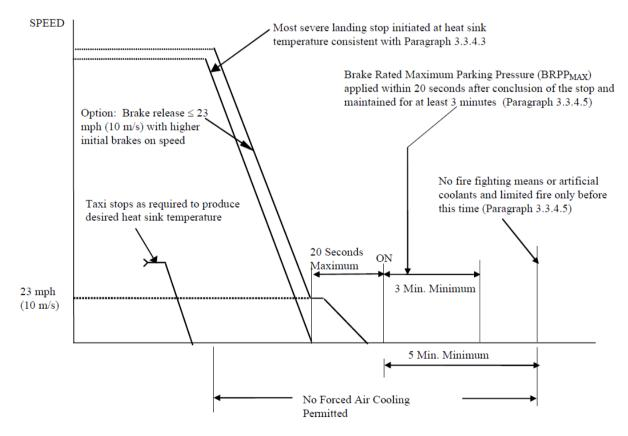
Figure 3-2. Most Severe Landing-Stop, Park Test Sequence
