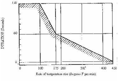
Figure 3 (a). Local temperature rise condition (Ref. Section 7.2.1)
