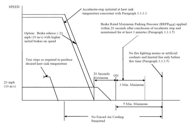
Figure 3-1. Taxi, Accelerate-Stop, Park Test Sequence
