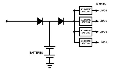
Figure A-2: An example BEPU Current Flow
