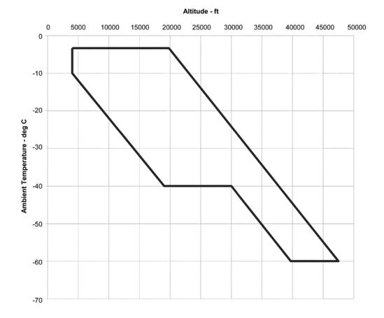
Within the envelope, total water content (TWC) in g/m3 has been determined based upon the adiabatic lapse defined by the convective rise of 90 % relative humidity air from sea level to higher altitudes and scaled by a factor of 0.65 to a standard cloud length of 32.2 km (17.4 nautical miles). Figure 2 displays TWC for this distance over a range of ambient temperature within the boundaries of the ice crystal envelope specified in Figure 1.
