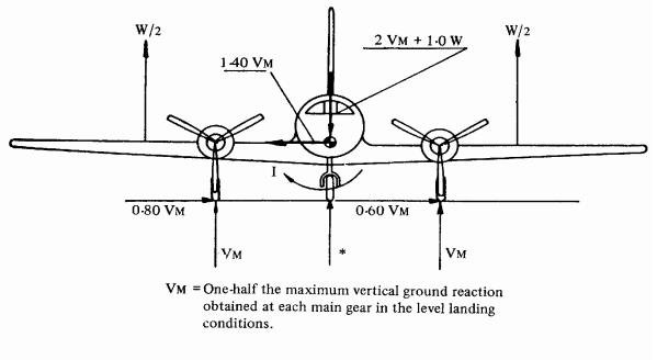
\*Nose-gear ground reaction = 0
