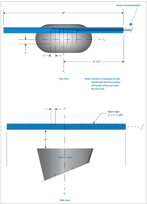
FIGURE 3 THERMOCOUPLE RAKE BRACKET
