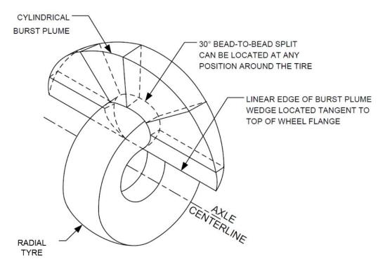
Figure 4e – Tyre Burst Pressure Effect – Radial Tyre
