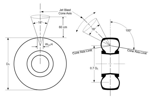
Note: 'Grown dimensions' should be calculated for bias tyres using TRA formulas.
