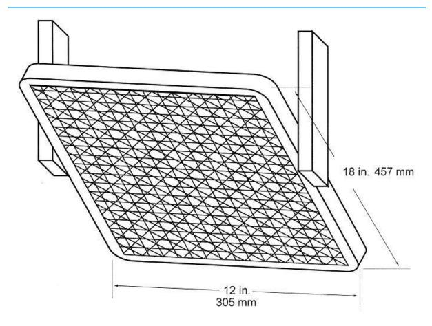
Figure 3b - Air Propane Radiant Panel
