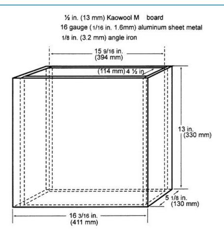
Figure 2 - Internal Chimney
