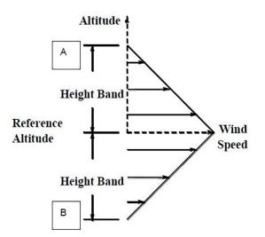
Note: The analysis should be conducted by separately descending from point "A" and climbing from point "B" into initially increasing headwind.
