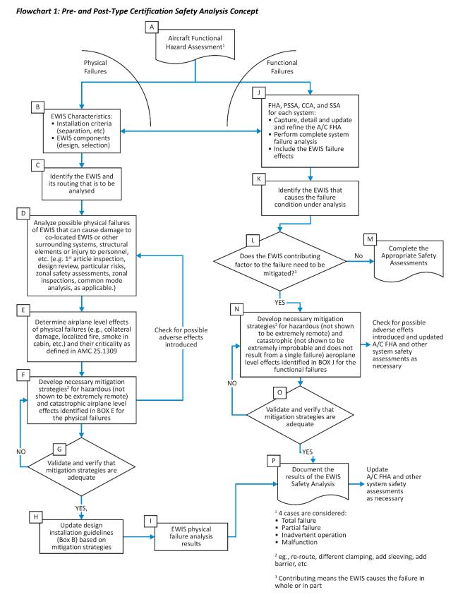
Note: Mitigation as used in this flowchart means to eliminate the hazard entirely or minimise its severity to an acceptable level.
