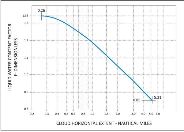
INTERMITTENT MAXIMUM (CUMULIFORM CLOUDS) ATMOSPHERIC ICING CONDITIONS VARIATION OF LIQUID WATER CONTENT FACTOR WITH CLOUD HORIZONTAL EXTENT Source of data – NACA TN No. 2738.
