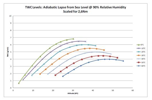
It is commonly recognised that below -40°C no liquid conditions exist anymore. Therefore testing in mixed phase conditions does not need to consider temperatures below -40°C.
