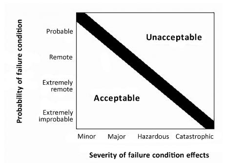
b. The safety objectives associated with Failure Conditions are described in Figure 2.
