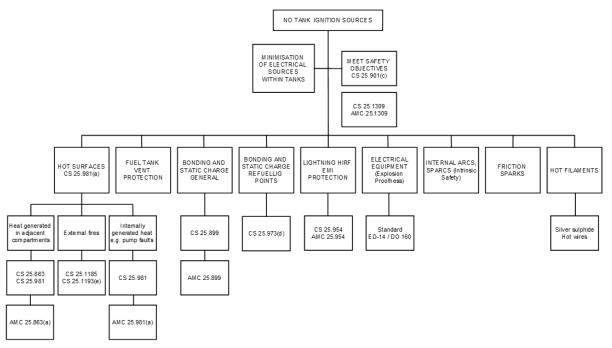
Therefore the focus of this evaluation of the aircraft fuel system should be to identify and address potential sources of ignition within fuel tanks, which may not previously have been considered to be unsafe features.
