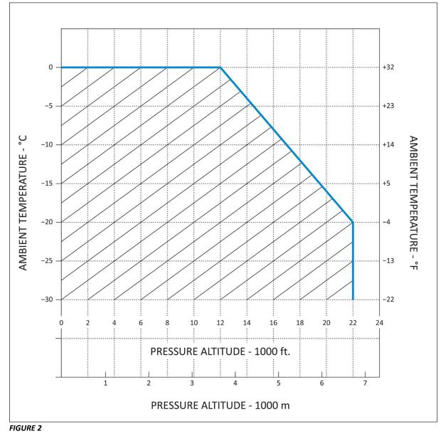
CONTINUOUS MAXIMUM (STRATIFORM CLOUDS) ATMOSPHERIC ICING CONDITIONS
