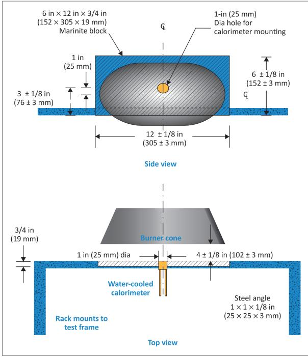
Figure 4 – Calorimeter Position Relative to Burner Cone
