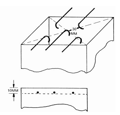
FIGURE 5. THERMOCOUPLE POSITION
