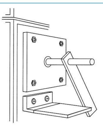
Figure 8 - Propane Burner Stop
