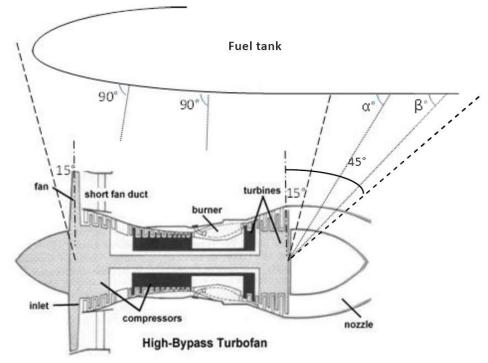
Note:  $\alpha$  and  $\beta$  angles are examples of possible angles between the fuel tank skin and the debris trajectory at the impact.
