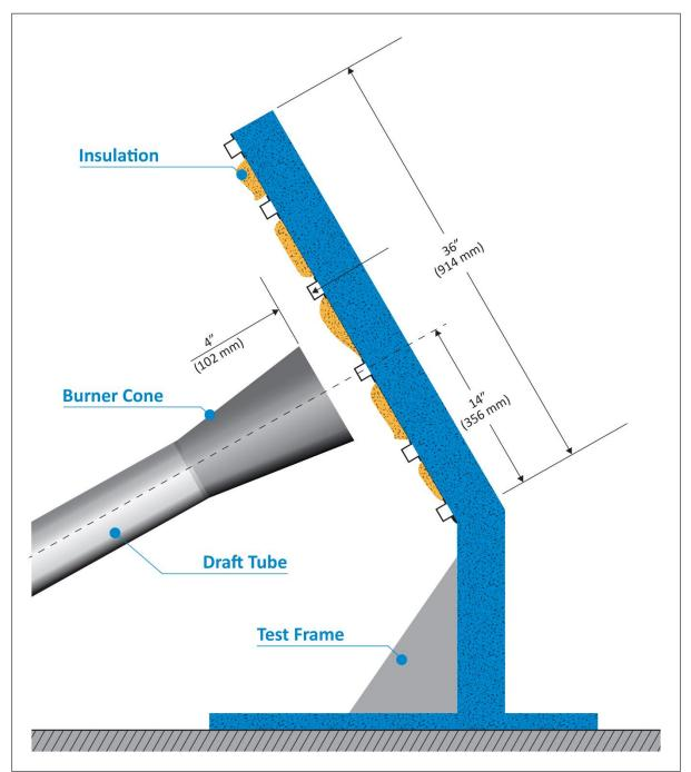
Figure 2 – Burnthrough Test Apparatus
