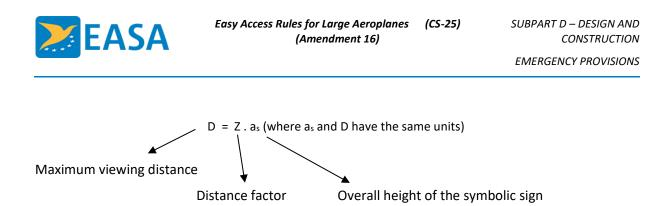
The maximum viewing distance "D" can be calculated from the overall height of the symbolic sign (as) by using the appropriate distance factor Z obtained from Table 1 below.
