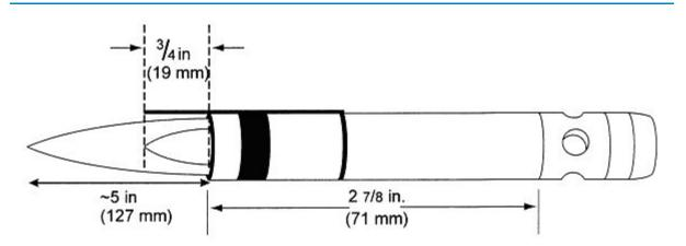
Figure 6 - Propane Pilot Burner
