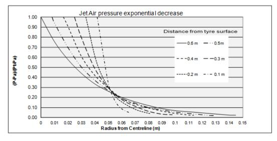
Pa= Ambient pressure P= P(x,z)= Pressure inside the cone as shown on Figure 2b Pt= Tyre Burst pressure
