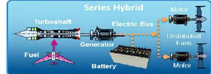
A system where only the electric motors are connected to the fans, and the gas turbine engine is used to drive an electrical generator which drives the motors and/or charges the batteries
