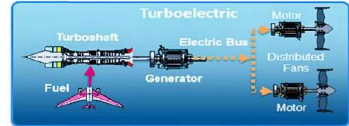
A system that relies fully on gas turbines to drive electric generators which then power inverters and motors to drive disturbed fans
