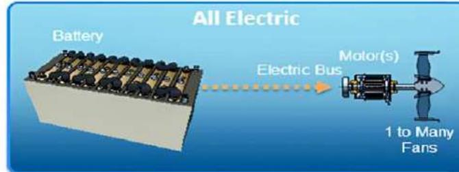
All-electric aircraft systems use batteries as the only source of propulsion power
