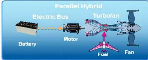
A system that uses a battery-powered motor and gas turbine engine both mounted on a shaft that drives fan, so one or both can provide propulsion at any given time
