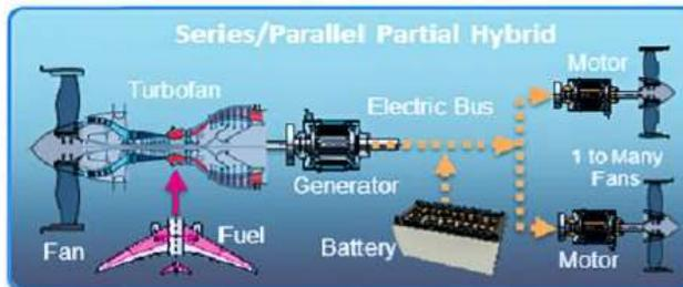
A system with one or more fans that can be driven directly by a gas turbine engine, and additional fans that are driven exclusively by electrical motors which can be powered by a battery or a turbine-driven generator
