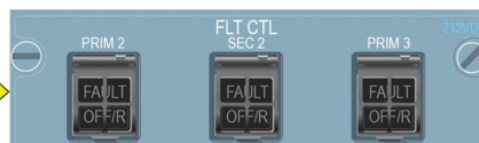
Example of pushbutton-switches on the overhead panel of an A330 aircraft
